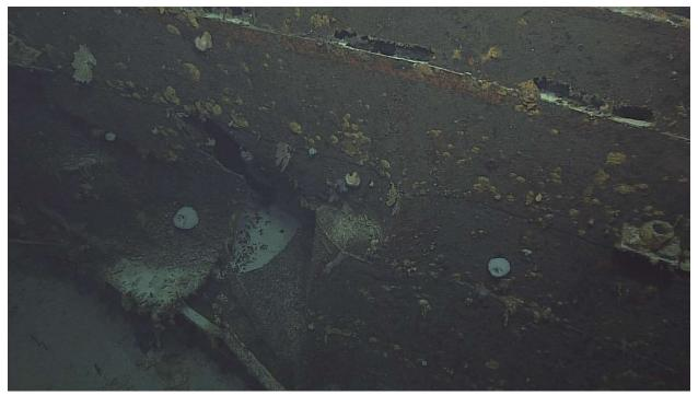
FIGURE 5.3. Lower aft hull damage most likely the result of a torpedo that struck the hull by USS *Triton* on 24 December 1942 leading to the vessel's sinking event (NOAA 2016b)
