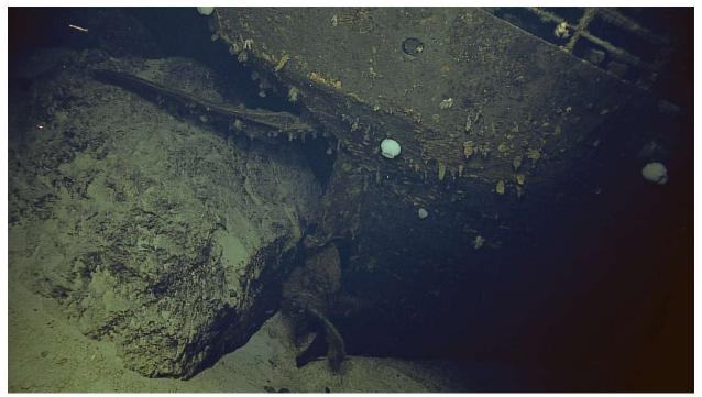
FIGURE 5.5. Rudder damage due to contact with boulder (NOAA 2016b)
