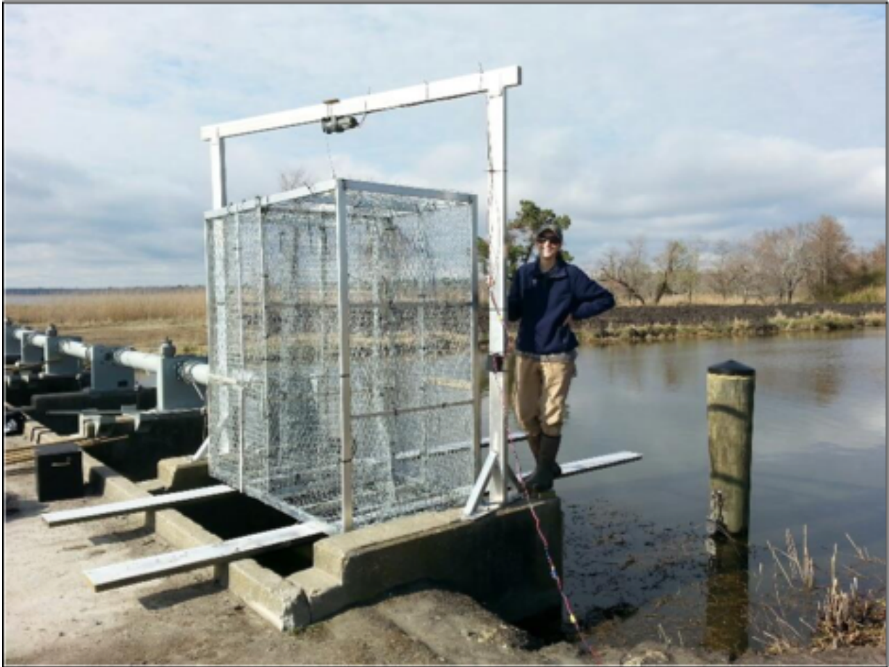
Figure 5. Photograph of Dr. Allison Stewart Mulligan alongside the winch system and the custom-built fish trap which was used in the side-hinged gates during the 2015 and 2016 field sampling campaigns at Waupoppin Canal, Lake Mattamuskeet, North Carolina (Mulligan 2020).
