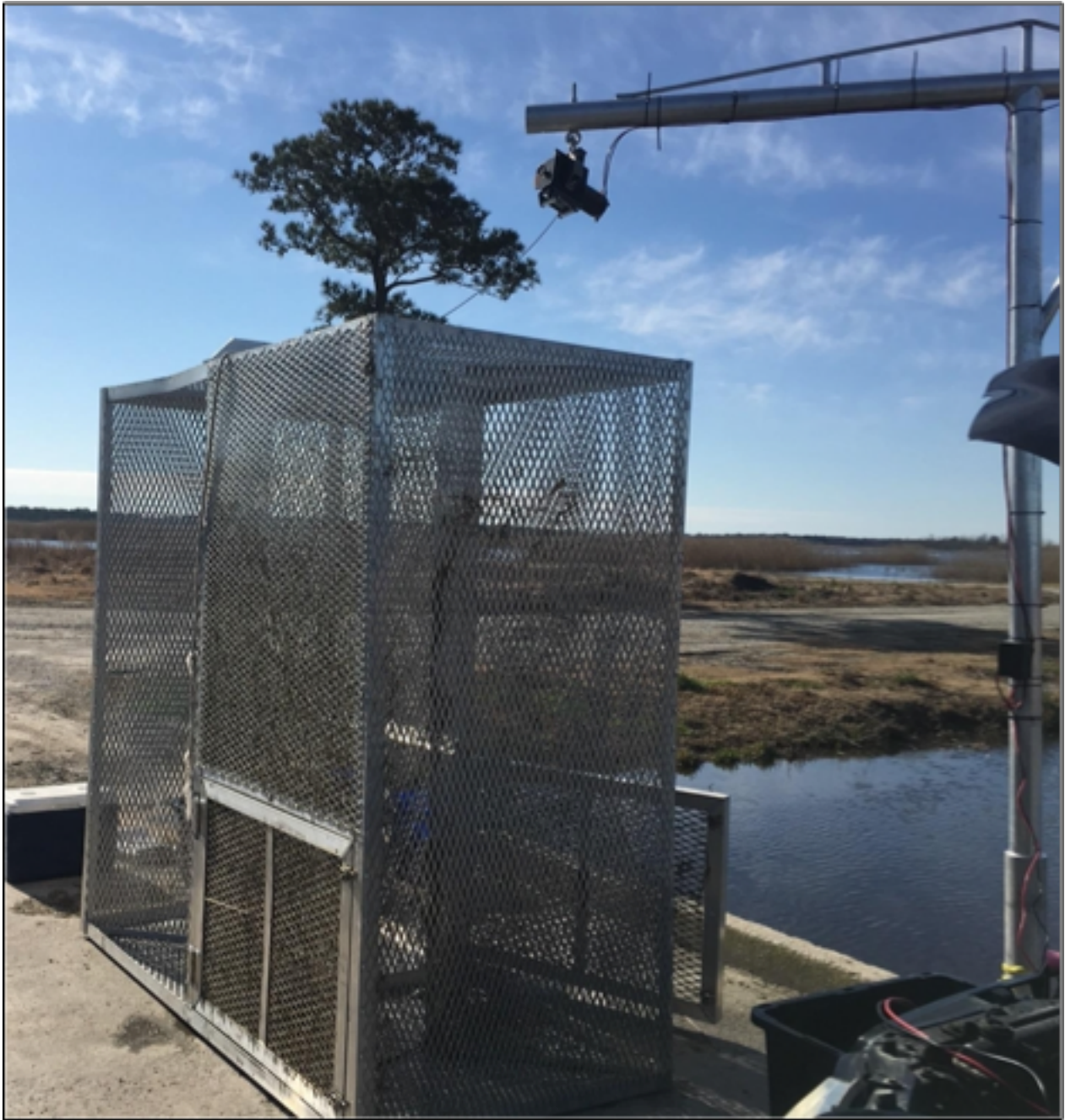
Figure 6. Photograph of the winch system and the custom-built fish trap which was used in the top-hinged gates during the 2016 field sampling campaign at Waupoppin Canal, Lake Mattamuskeet, North Carolina (Mulligan 2020).
