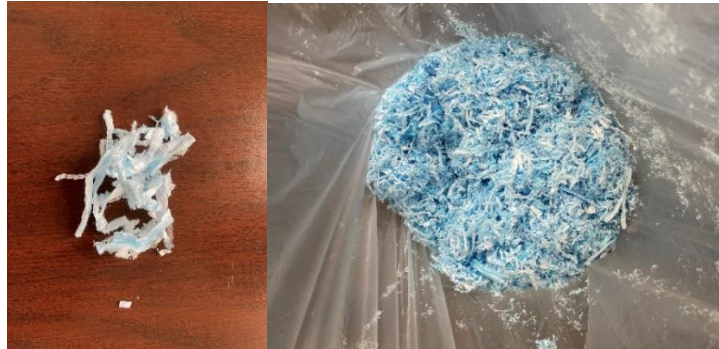
Figure 3.3: Shredded Face Masks to Be Added in the HMA Mixes as a Modifier
