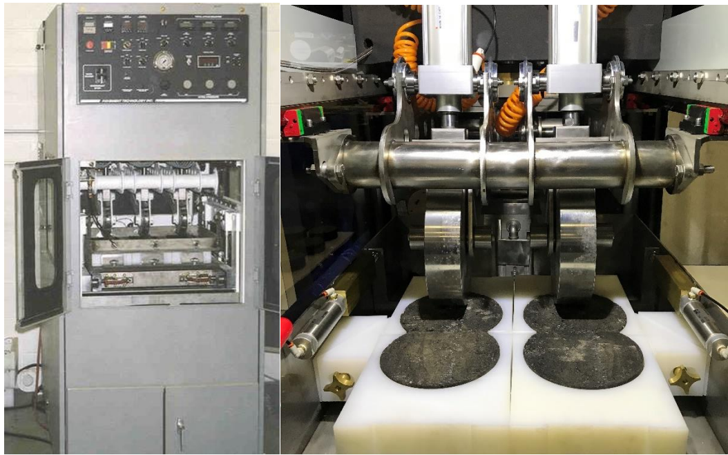
Figure 3.6: APA Machine and Test Samples in APA Chamber
