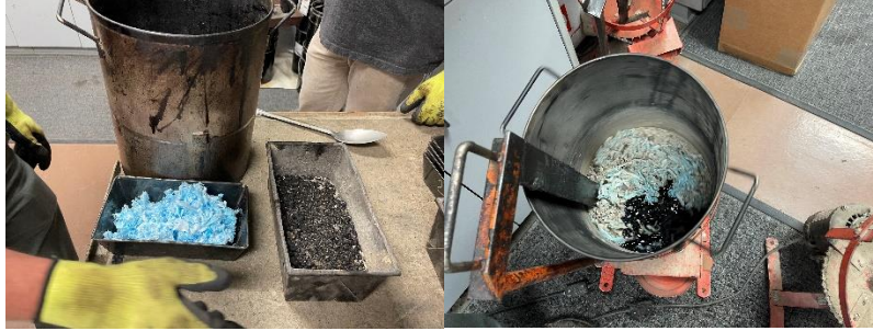
Figure 3.5: The Shredded Face Mask (SFM) with HMA Virgin Materials and Reclaimed Asphalt Pavement (RAP)
