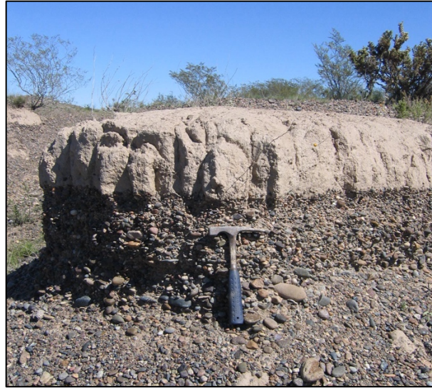
Figure 24. Harsh erosional base between the alluvial gravels and overlying eolian unit (copyright permission, H. Luchsinger).
