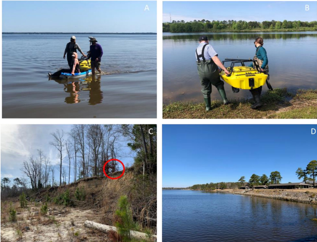
Figure 14. Challenges while using the sUSV in shallow nearshore bathymetric environments. A: Shows the use of three crew members transporting the sUSV through the shallow water. Two crew members to stabilize the sUSV and move the kayak, and one to balance the weight on the kayak. B: Two crew members carrying the sUSV into the water. C: A survey location where the shoreline bluffs of 15 m in elevations and pine tree cover caused RTK-GNSS error. The red circle shows the location of the base station. D: Ideal wave conditions, waves light chop and winds <10 kts, at YMCA Camp Seafarer.
