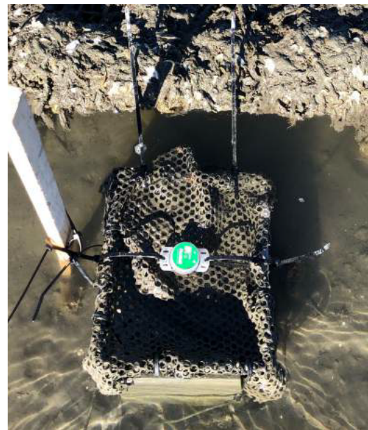
Figure 3. Landward passive sampler with a HOBOTemperature logger connected to the top. Photo credit: Rachel Gittman
