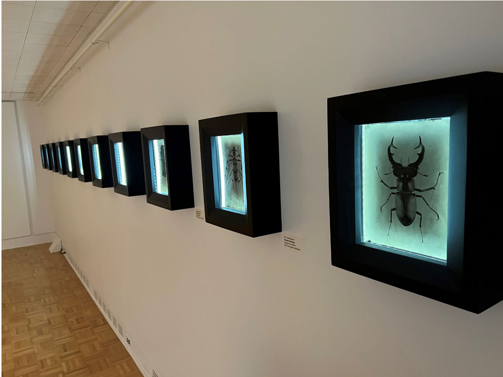
Figure 9. View of one wall in the gallery. Power cords are not visible for each of the works. Power is supplied via copper foil tape that is affixed to the wall and painted over.
