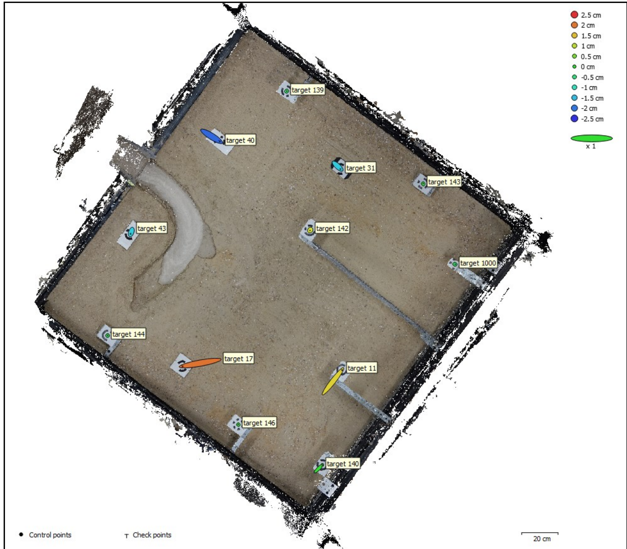
Figure 17. Visualization of GCP displacement from experiment start to finish. Check points and control points mark GCP positions during the final trial; shape of error trail shows distance traveled since first trial.
