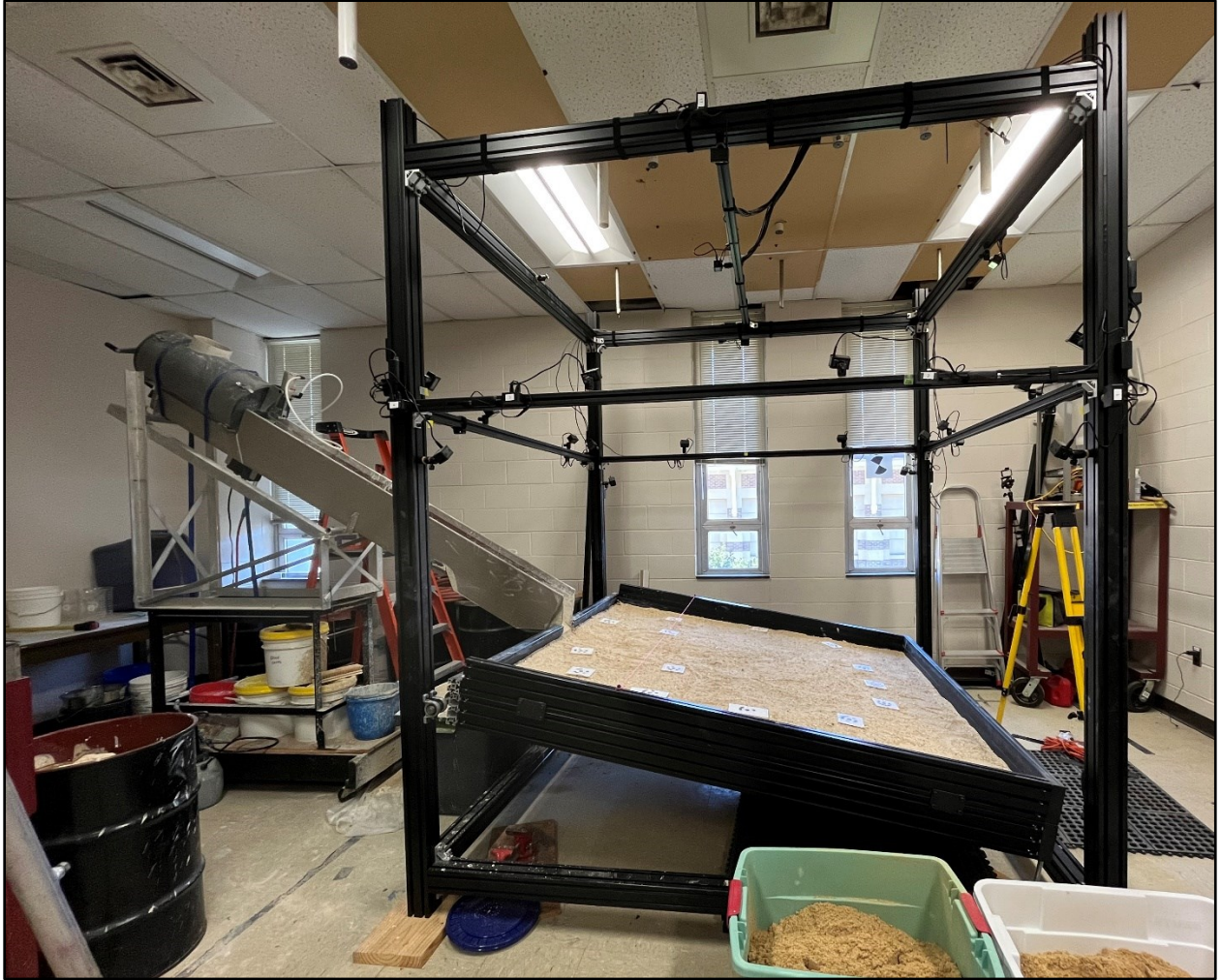
Figure 2. Photo of the debris-flow modeling flume situated in the ECU Geomorphic Modeling Laboratory.
