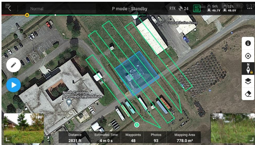
Figure 22. UAS Flight Plan for the West Water Treatment Building
