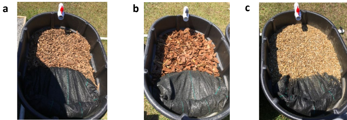
Figure 3.2 Images of uncovered bioreactors demonstrating the various denitrifying media (a) woodchips, b) pine bark, c) peanut hulls). The denitrifying substrate comprises the upstream end of the bioreactor (closest to the influent pipe), and the expanded slate (encased in a geotextile sack) comprises the downstream end.
