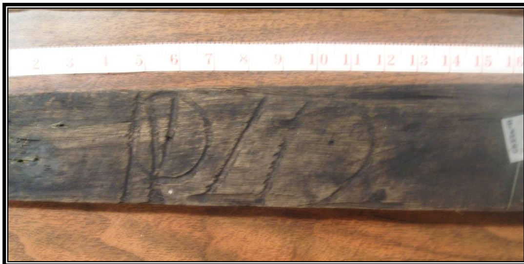
FIGURE 1.4. A stave recovered from the Betsy showing possible maker's, shipper's marks, assembly marks, and graffiti from the late eighteenth century (the scale shown above is in inches). (Photo by author 2006.)
