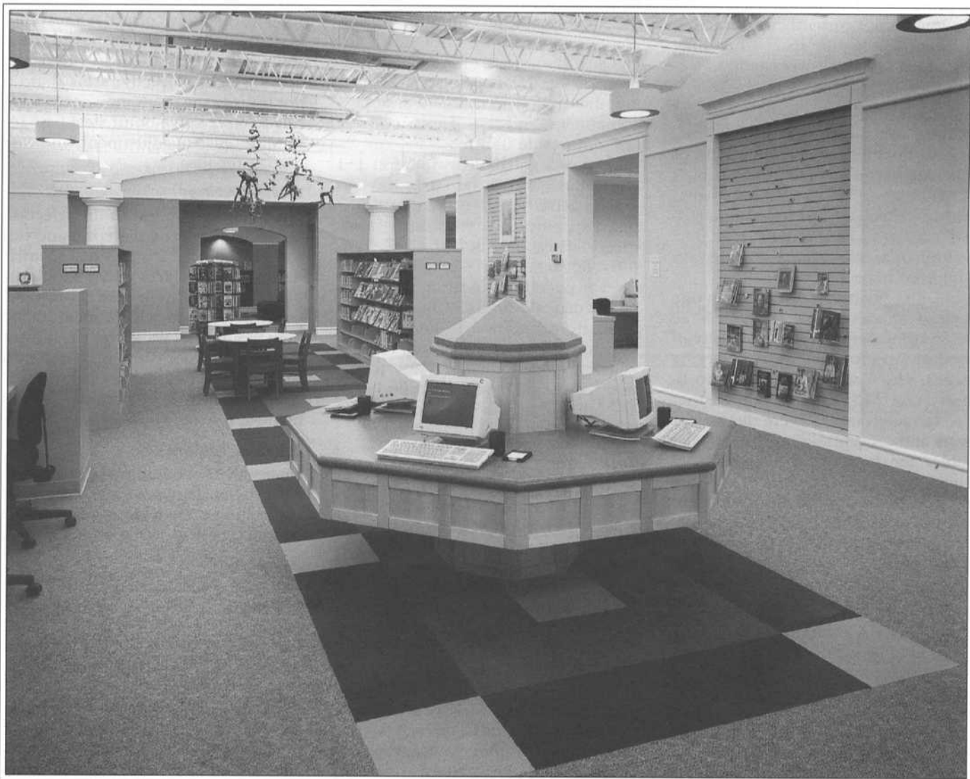
The Independence Regional Library of the Public Library of Charlotte and Mecklenburg County utilizes a hexagonal-shaped computer workstation which effectively conceals the power and data wiring. Library materials are displayed using slotwall panels. Architect: TBA 2 Architects (Charlotte) Photo: Ciarlante.
