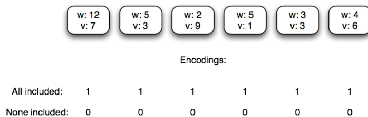
Figure 2.12: Simple encoding scheme for genetic algorithm knapsack problem optimization. Items represented by a 1 are included, and those with a 0 are not.
