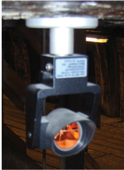
Figure 3-3: A fixed prism mounted on the lower gundeck.
