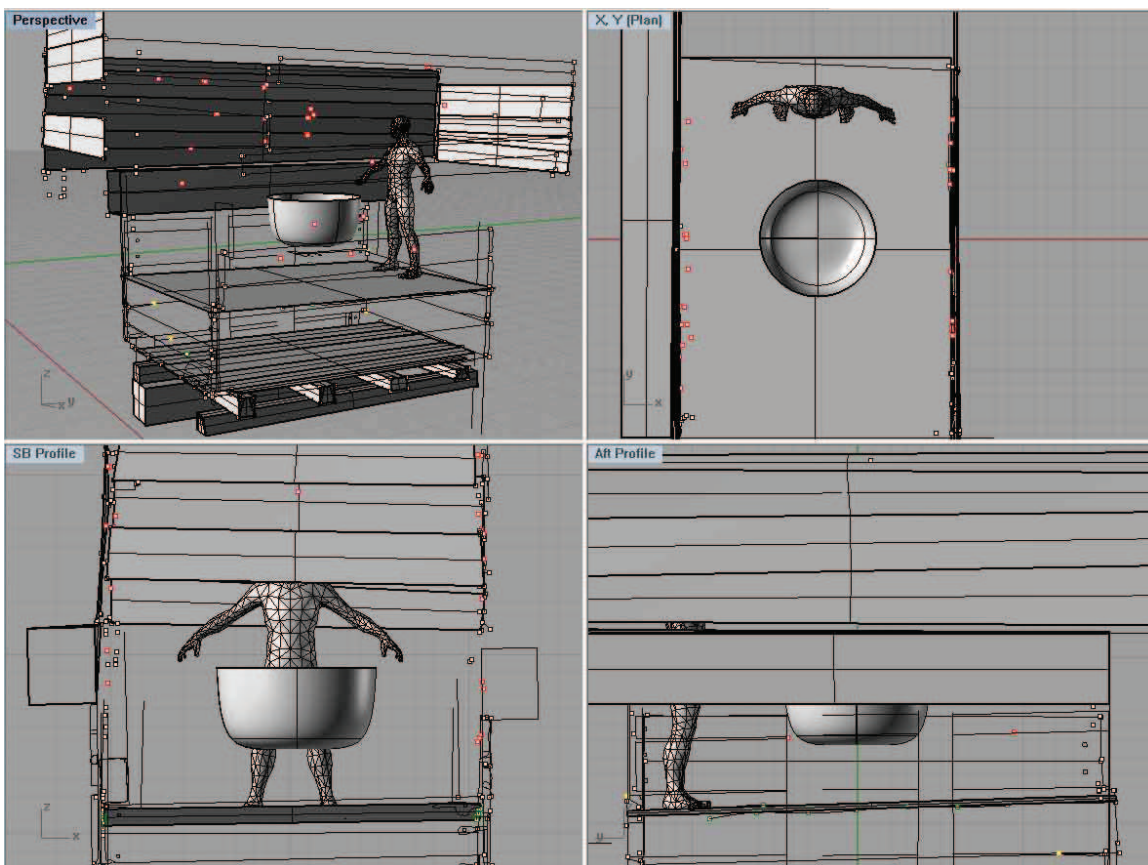
Figure 5-15. This screenshot from Rhinoceros shows the galley model in progress. As can be seen, the digital cook stands at a representation of Vasa's iron cauldron.
