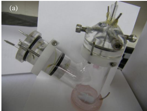
Fig. 3-13 (a) A photo of the integrated sample reservoir, stirrer and flow chamber. Slave piston is at left near bottom of side arm of Y shaped vessel. (b) The schematic of the assembly with flow chamber at top (green). Injector needle steering screws are around top of reservoir just below supply and injector tubes. Sheath and core are fed in through two small tubes flanking injector needle. Magnetic stirrer is at bottom with provision for draining reservoir.
