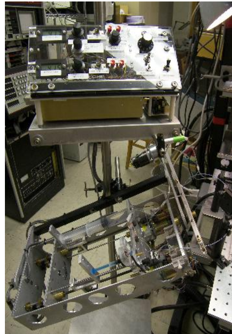
Fig. 3-5 The three-channel syringe pump. Entire drive assembly (at bottom) undergoes rocking motion to keep suspensions from settling and is tilted up when removing bubbles.
