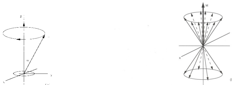
Figure 7. (a) Precession of \mu about B_0 ; (b) Precession of an ensemble of nuclei with I=1/2
