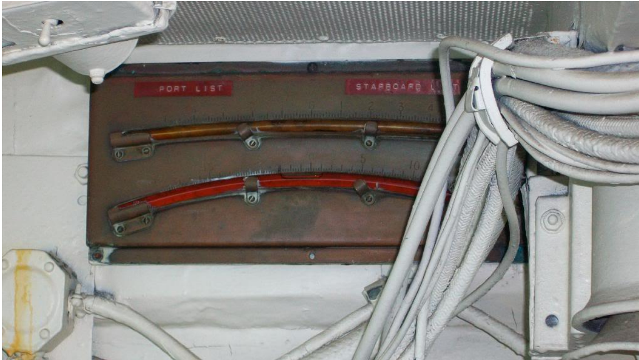
Photograph 65: Measurable indication the Lexington is listing.
