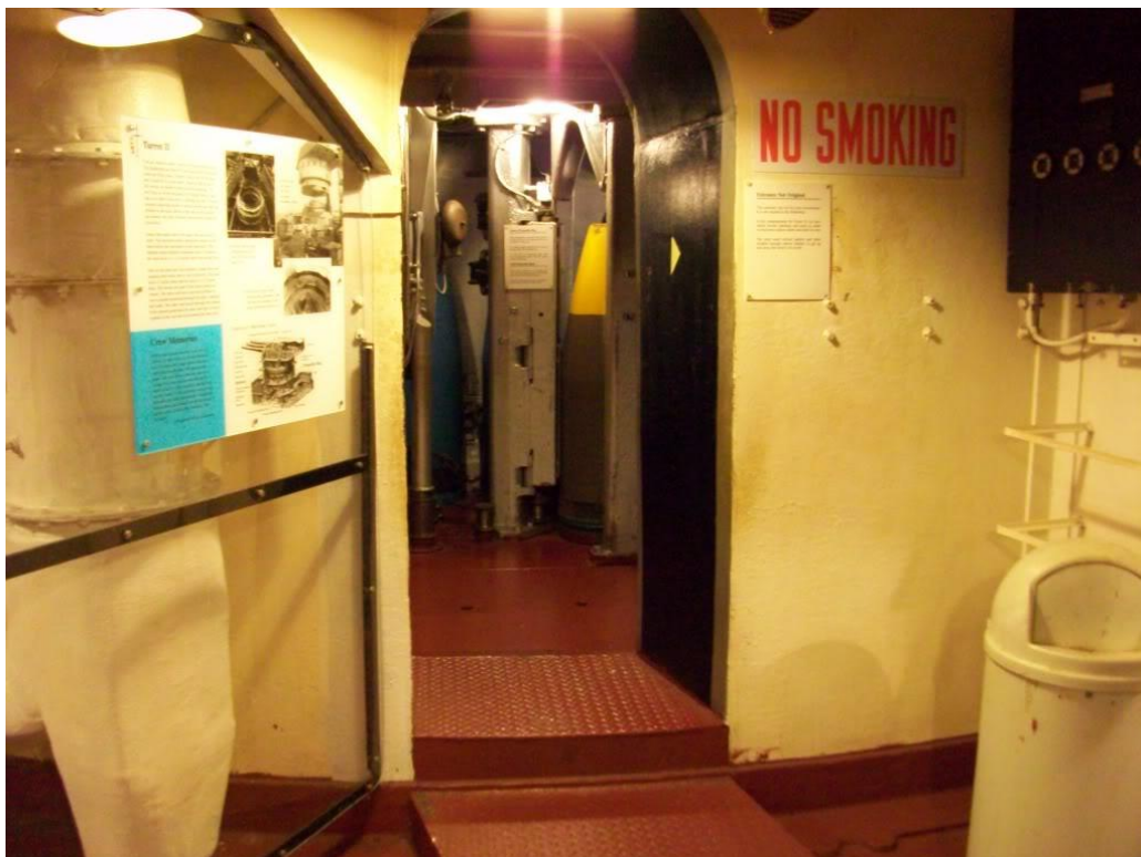
Photograph 15: Entryway cut through magazine armor below Turret #2.
