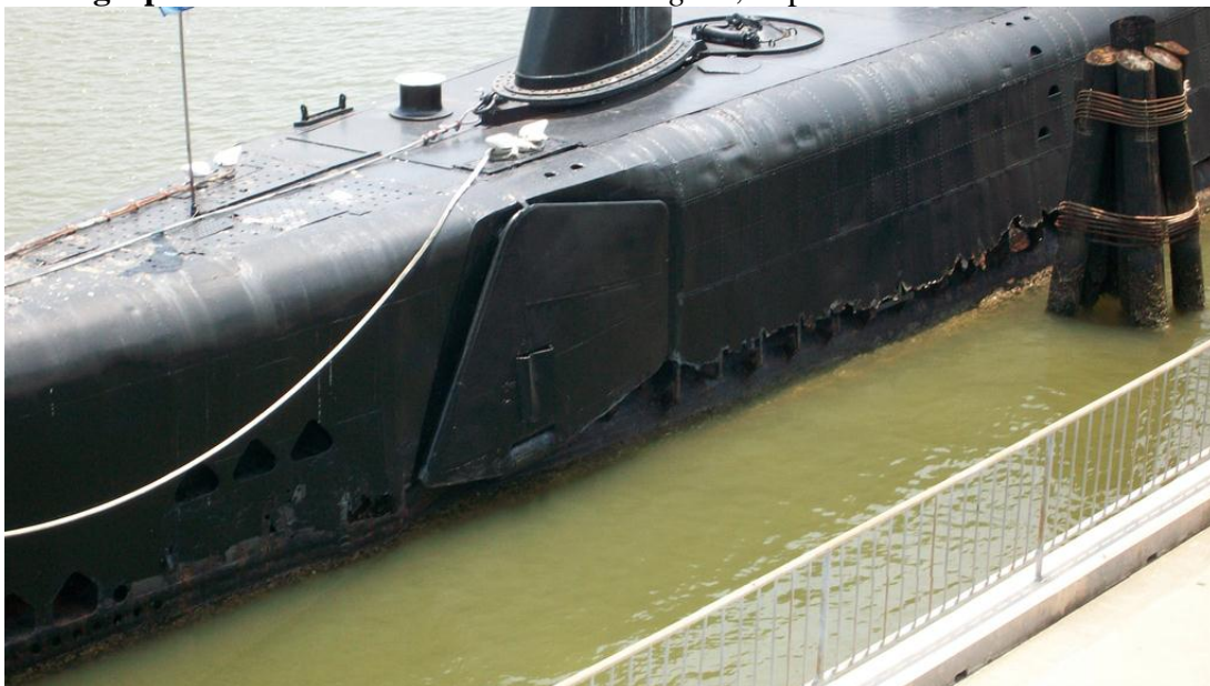
Photograph 54: Corrosion on Clamagore's hull, June 2009.
