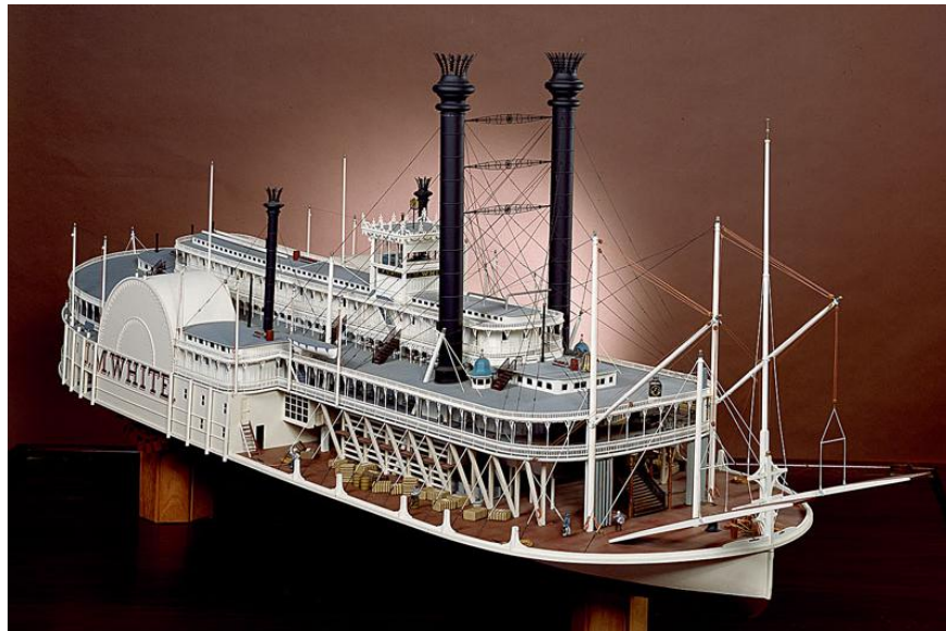
FIGURE 14. Model of the side paddlewheel, cotton packet J. M. White , built in Jeffersonville, Indiana, in 1878, for the Greenville and New Orleans Packet Company. Note the protruding stem post on the model bow and the landing stage (Smithsonian National Museum of American History 2011).
