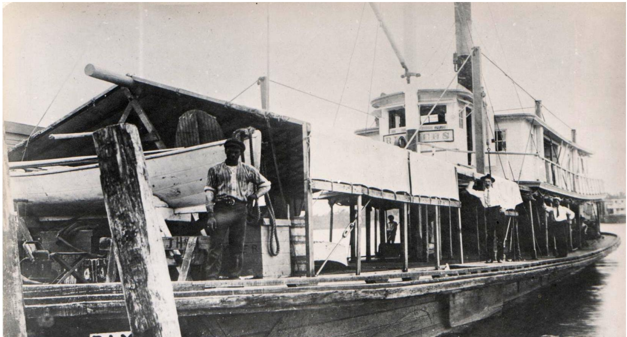
FIGURE 37. Photograph of upriver steamboat R. L. Myers (II) , note the tented versatile main deck and the passenger saloons on the upper deck (Courtesy of Bridgers Collection, Outer Banks History Center).
