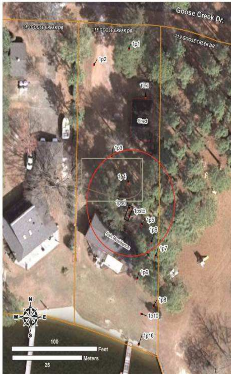
Figure 5. Site map of Site 1. Piezometers/Well clusters are indicated by the red dot. Drainfield area is represented by a box north of the OWTS (1sto/1sti). Red circle represents the approximate 15 meter (50 ft) setback radius from D-box location in accordance with North Carolina State rules 15 A NCAC 18A .1950.
