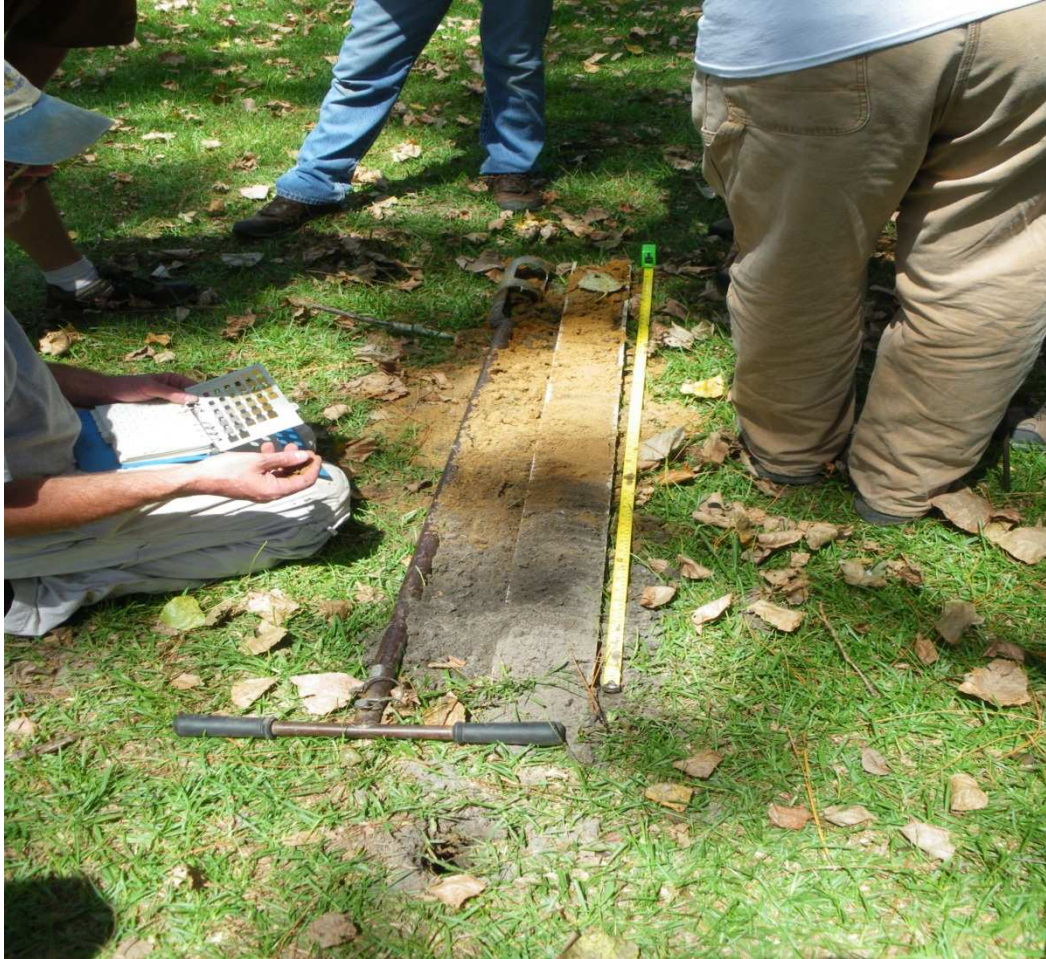
Figure 3. Soil profile of soil taken from drainfield at Site 2. The first 90 cm consist of predominantly sandy soils. A layer of sandy loam is present at depths between 90 and 125 cm. (Humphrey, 2010).
