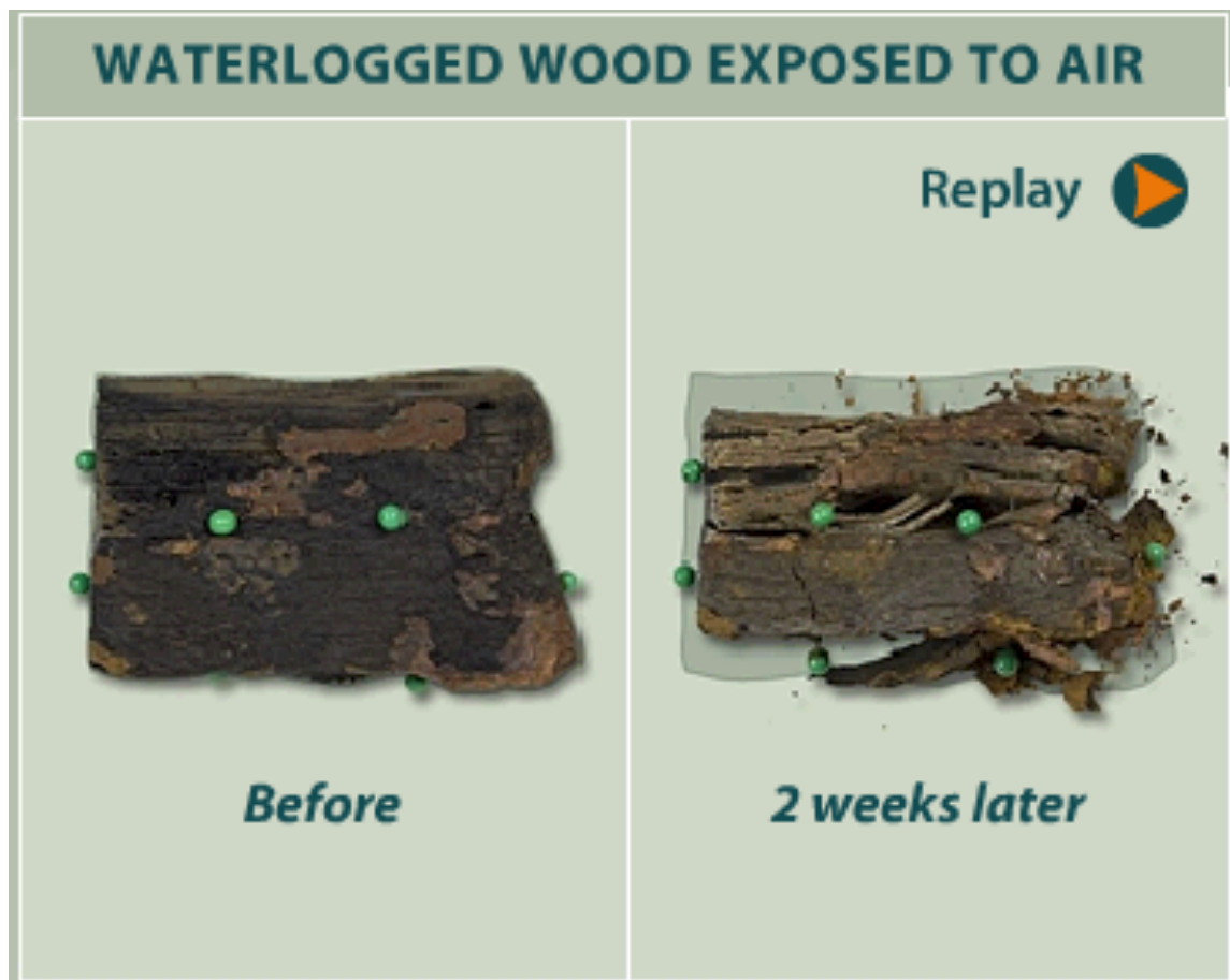
Figure 1. A screen shot from a video depicting the structural damage caused by uncontrolled drying of waterlogged wood. Image courtesy of the Mariners' Museum.
