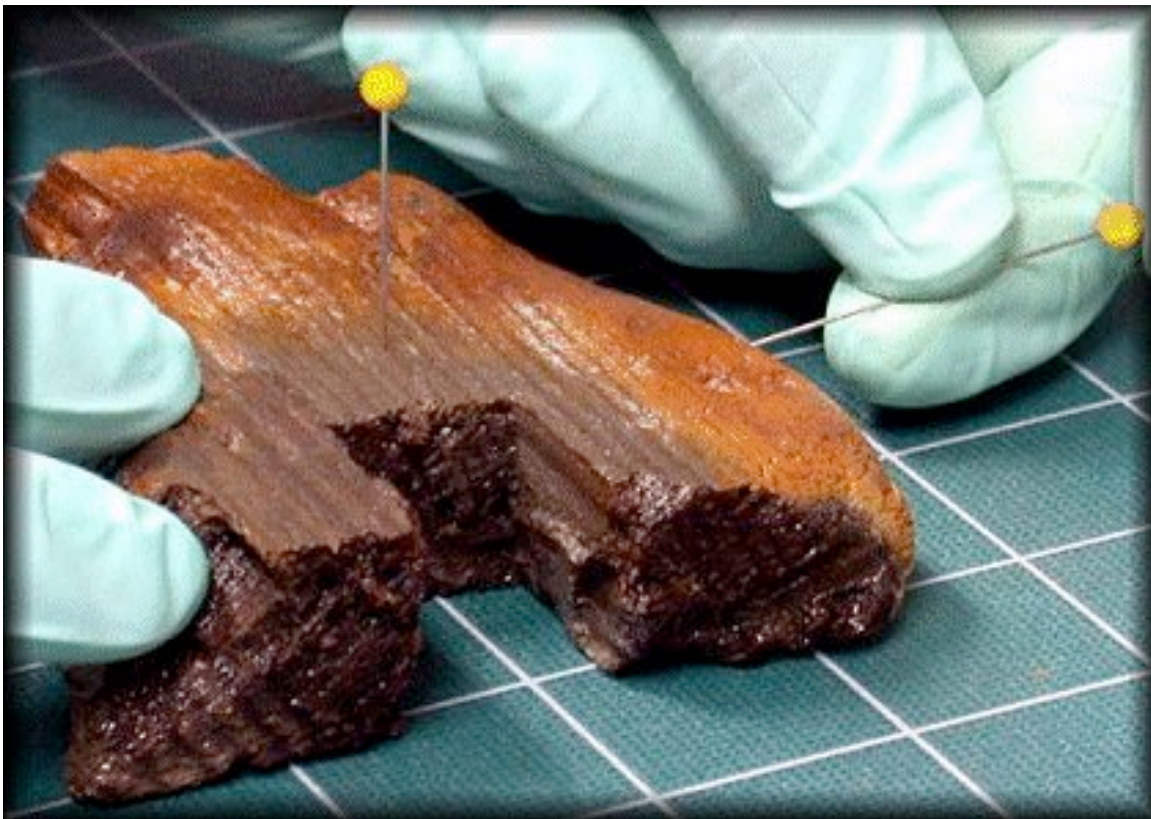
Figure 11. An image provided by The Queen Anne’s Revenge Conservation Laboratory located at East Carolina University of the pin test being performed by a conservator.
