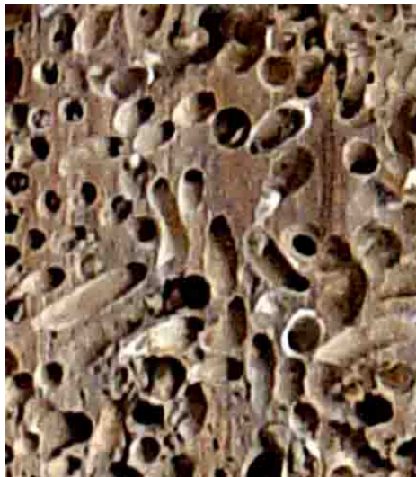
Figure 2. Teredo worms are bivalves that can live on wood and are a primary threat to wood stability in a marine environment.
