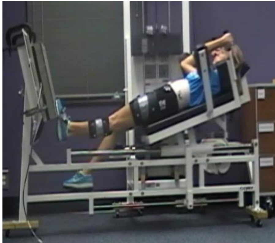
Figure 2: Subject setup on the Cybex Leg Press Machine used for torque-velocity tests and strength training.
