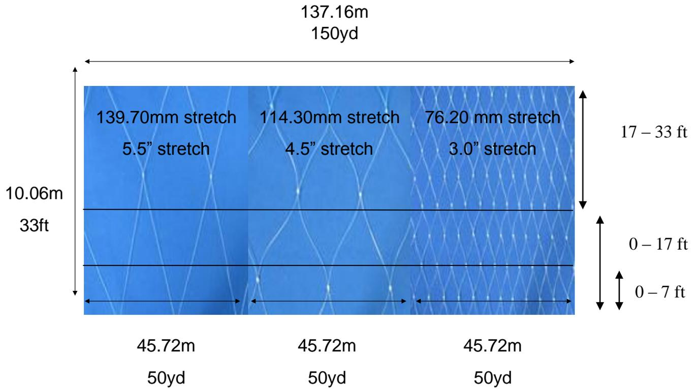
Figure 11. Dimensions of the vertically elongated gillnet illustrating mesh size and panel size used to estimate the location of spiny dogfish suspended in the water column.
