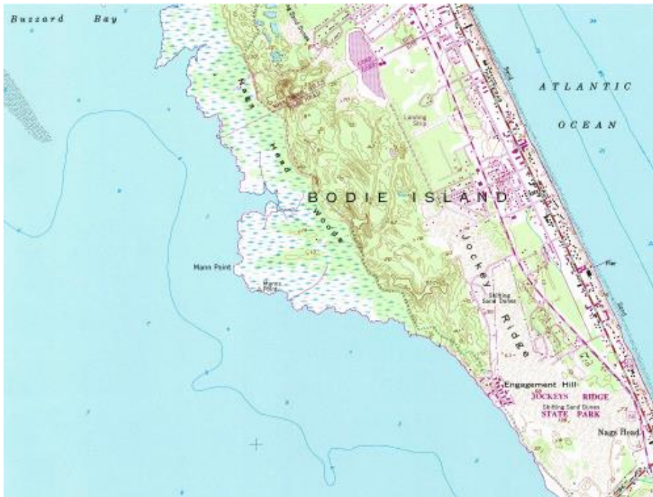
Figure 6.7 USGS topographic map highlighting contour lines (USGS 2012).
