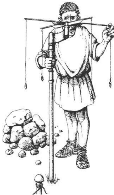
Figure 2.6 A Roman survey instrument, the groma ( http://www.the-romans.co.uk ).
