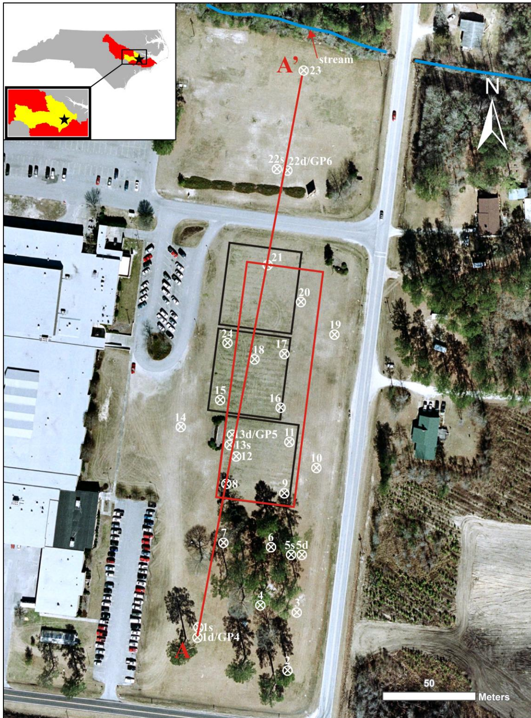
Figure 3. Site map of study area at WCHS. The active wastewater drainfields are represented in black along with the inactive drainfield to the north. The geophysical survey area and transect are represented in red. Piezometer, surface water sampling points, and core locations are shown. Core locations are indicated by GP. Aerial photo is from Google Earth (2012).
