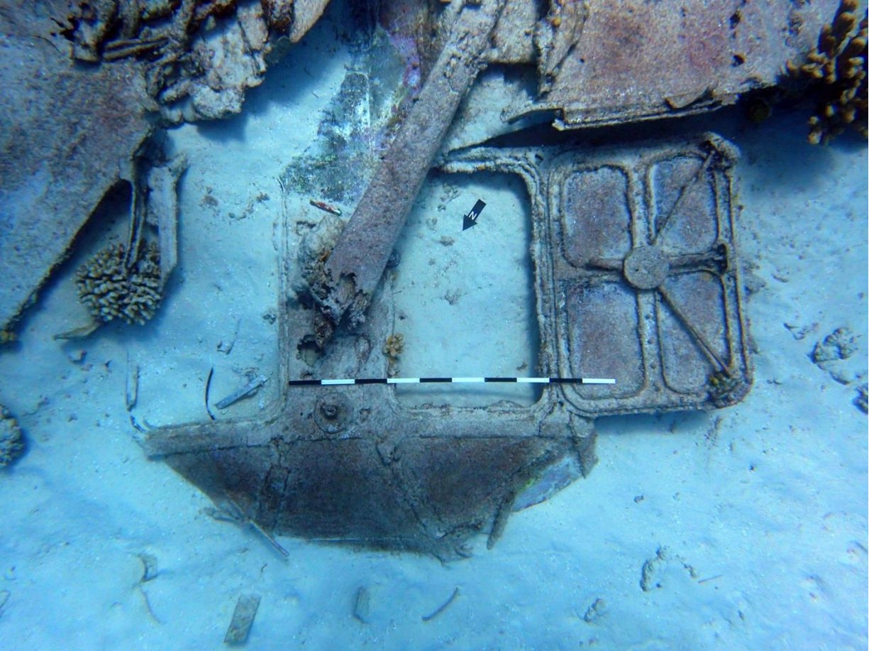
Figure 22. Feature 1. Cockpit canopy windows, pilot's escape hatch, and aerial mast. Plan view, 1 m scale.
