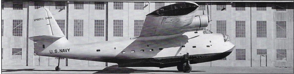
Figure 7. Original XPB2Y-1 tail configuration with single vertical stabilizer (Consolidated).
