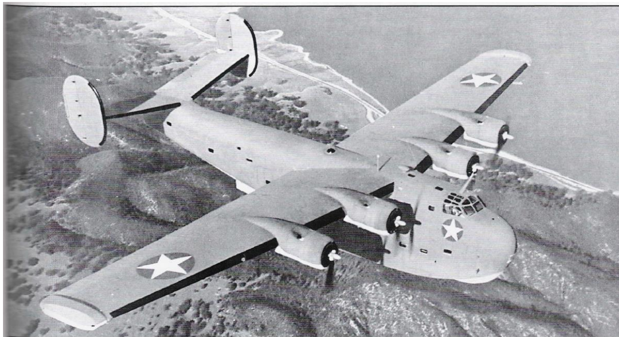
Figure 12. PB2Y-3R transport conversion. All guns have been removed (Consolidated).
