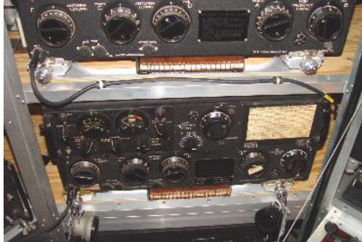
Figure 25. Contemporary ART-13B transmitters from B-29 flight deck (Photograph aafradio.org).
