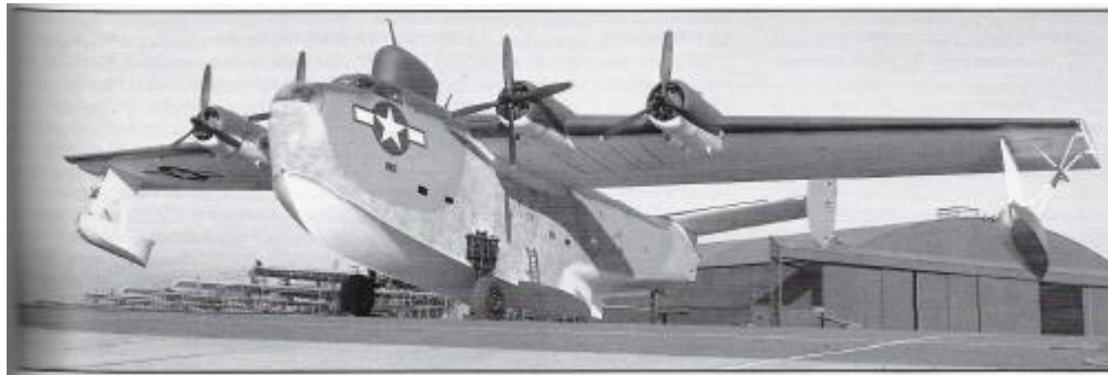
Figure 13. PB2Y-5 with radome installed above flight deck (US Navy).
