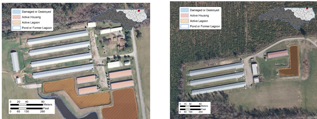
Figure 20: Two examples of poultry CAFO buildings in very close proximity to swine CAFO buildings. Only the swine CAFO housing and lagoons are delineated and classified. Aerial imagery from 2013, provided by the NC One Map service.
