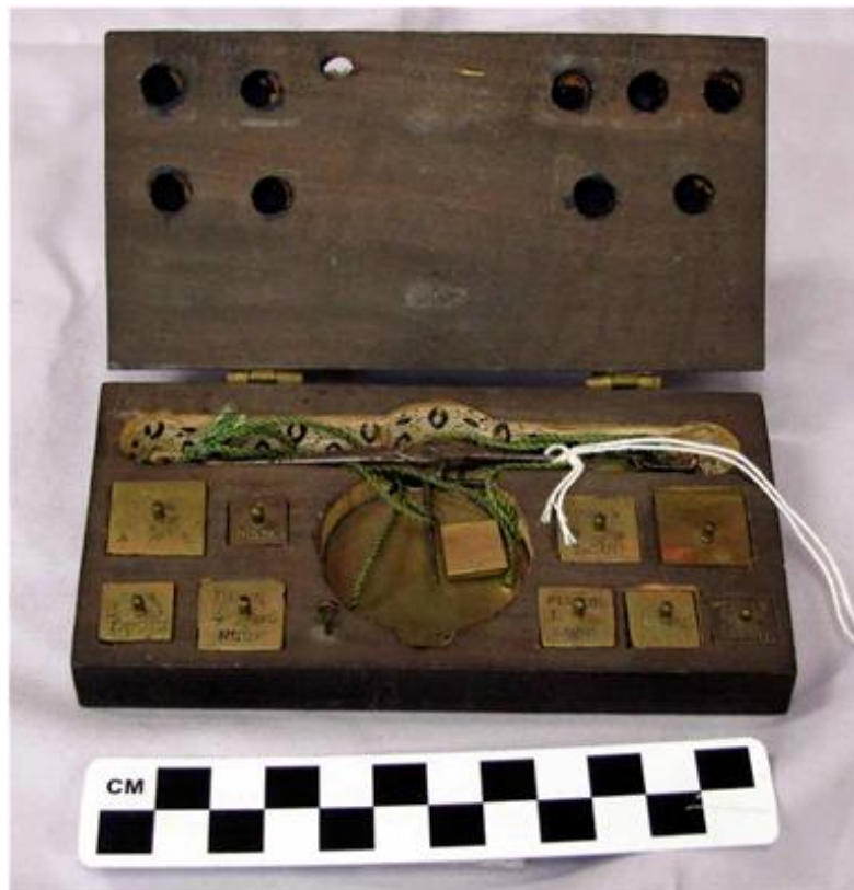
French hand balance with weights and case. (Courtesy of The Mütter Museum, Philadelphia, PA.)
