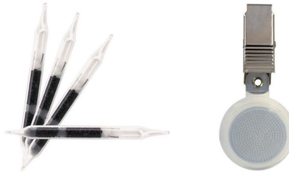
Figure 2. Activated charcoal tubes and diffusive samplers
