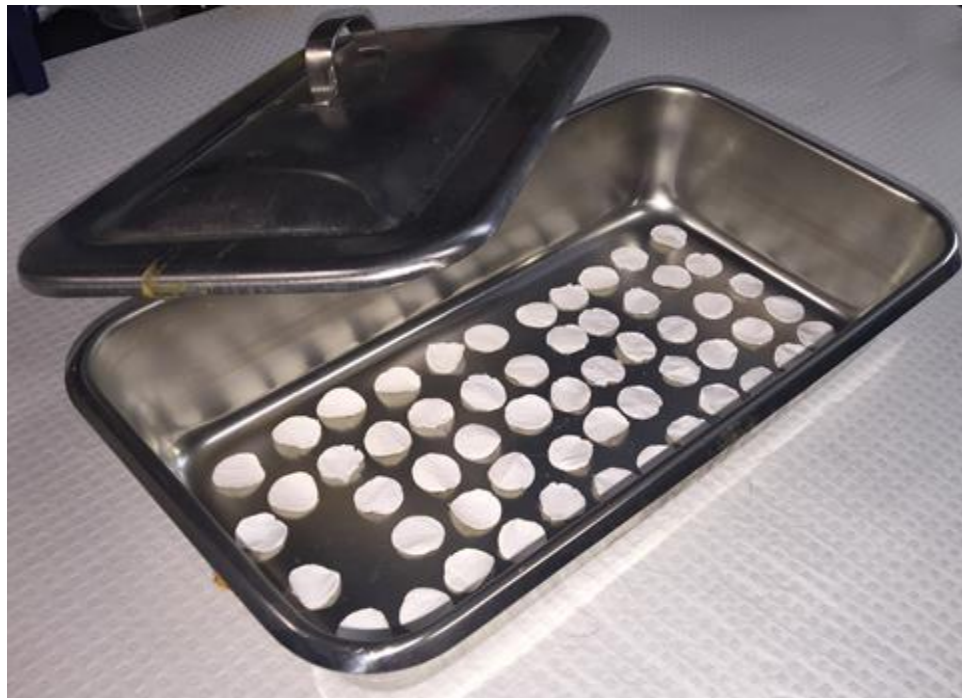
Figure B.2: Scaffold arrangement for crosslinking
