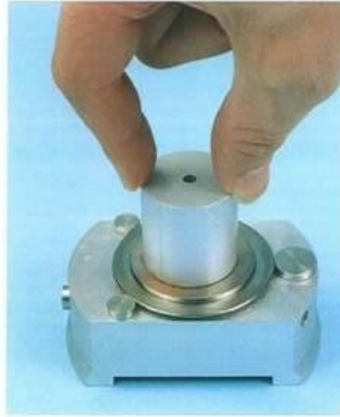
Figure B.4: Pressing Powder with Powder Press Block
