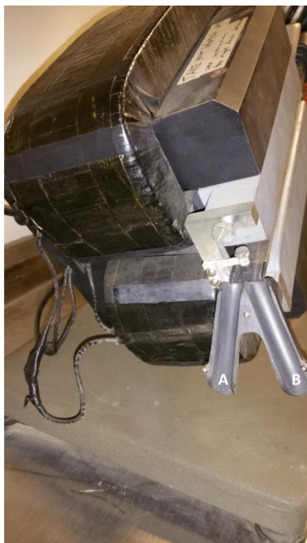
A = Nonmagnetic Sediment Chute B = Magnetic Sediment Chute
