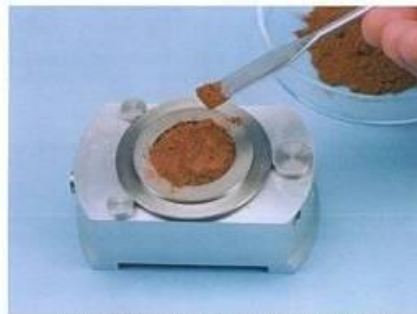
Figure B.3: Spreading Powder in Sample Holder Ring
