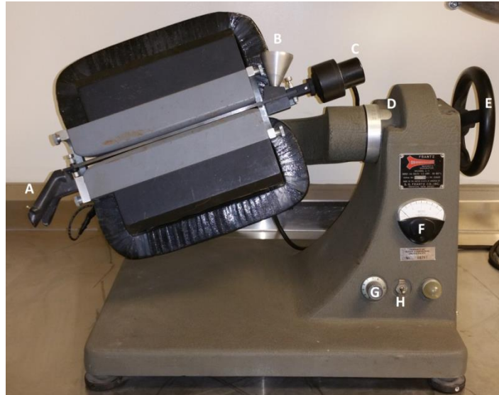
A = Chutes B = Sediment Funnel C = Slide Vibrator D = Side Slope Angle E = Side-Slope-Adjuster Wheel F = Amp Meter G = Slide-Vibrator-Adjustment Knob H = Slide-Vibrator-Power Switch
