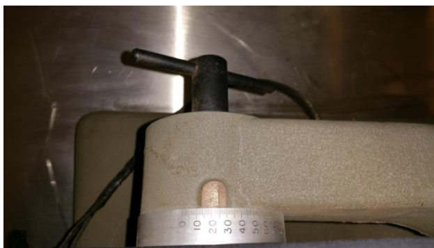
Forward-Slope-Angle Adjustment Knob (Located in the back of the Frantz Magnetic Separator)
