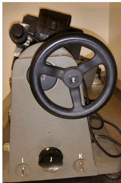
E = Side-Slope-Adjuster Wheel I = Hi/Low Power Switch J = Magnetic-Coil-Amperage-Adjuster Knob K = Power Switch for Magnetic Coil
