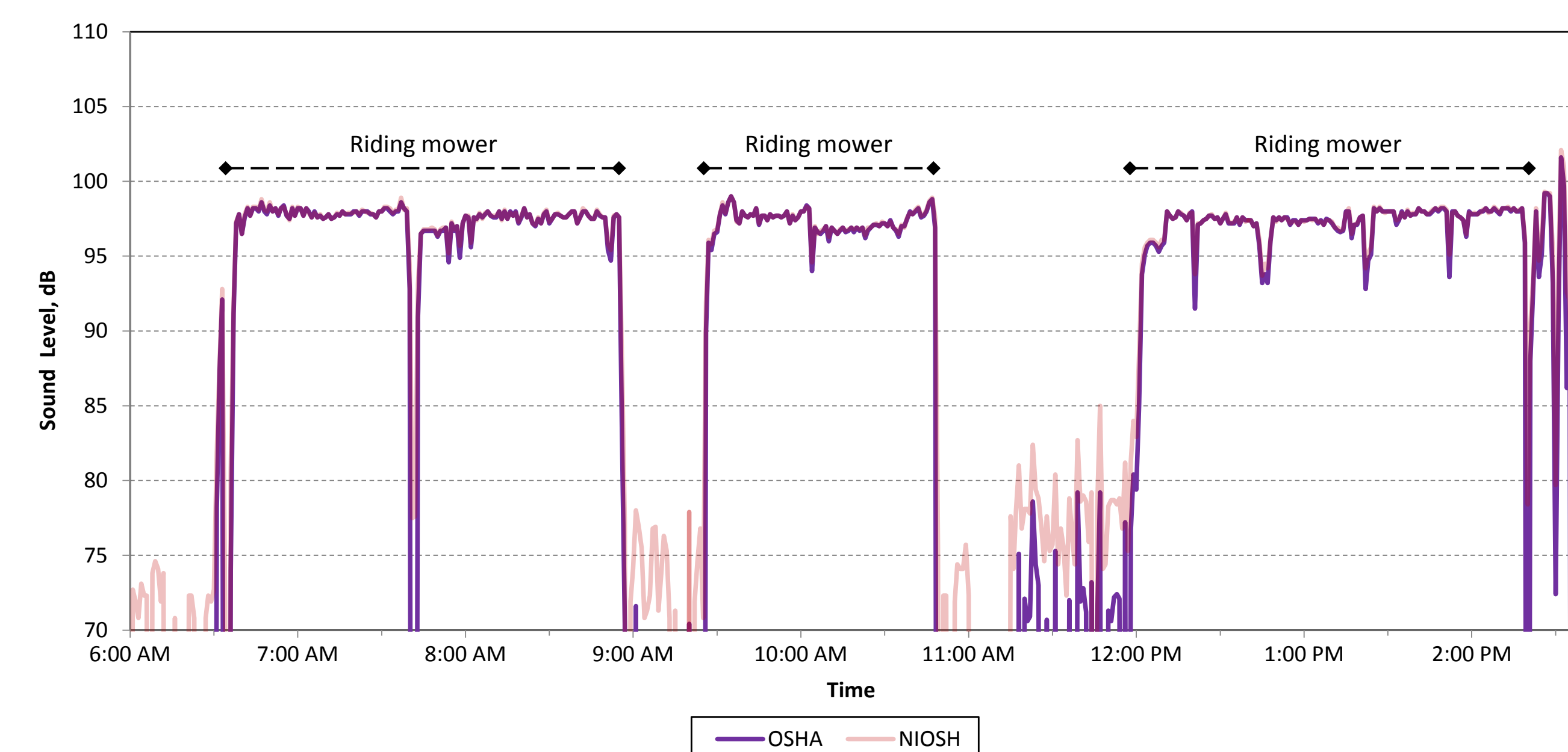
Figure 7. Noise exposure profile of a UnivB groundskeeper with 8-hr OSHA TWA = 95.5 dBA (highest TWA among riding mower users)
