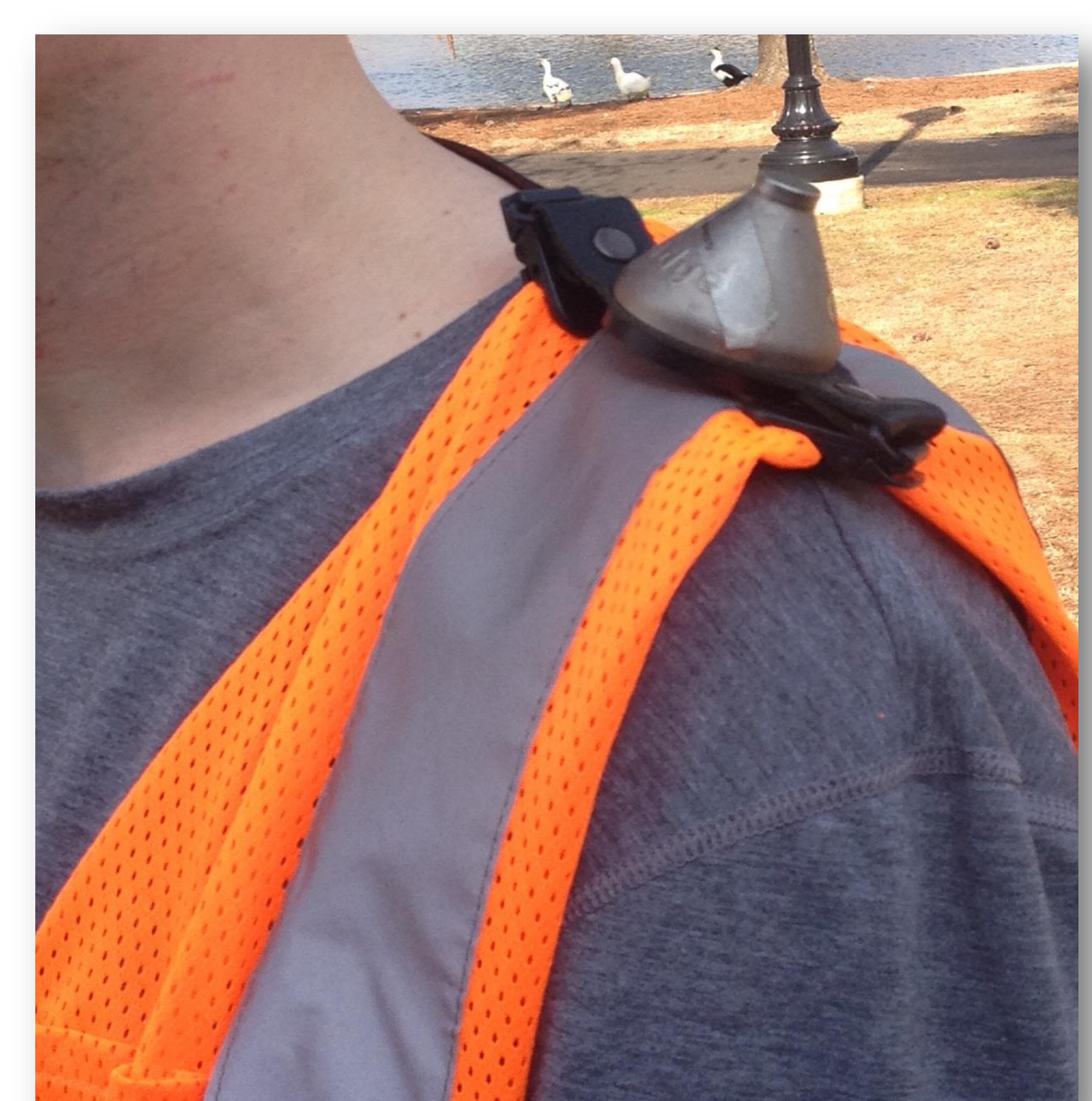
Figure 1. Noise dosimeter worn by a groundskeeper
