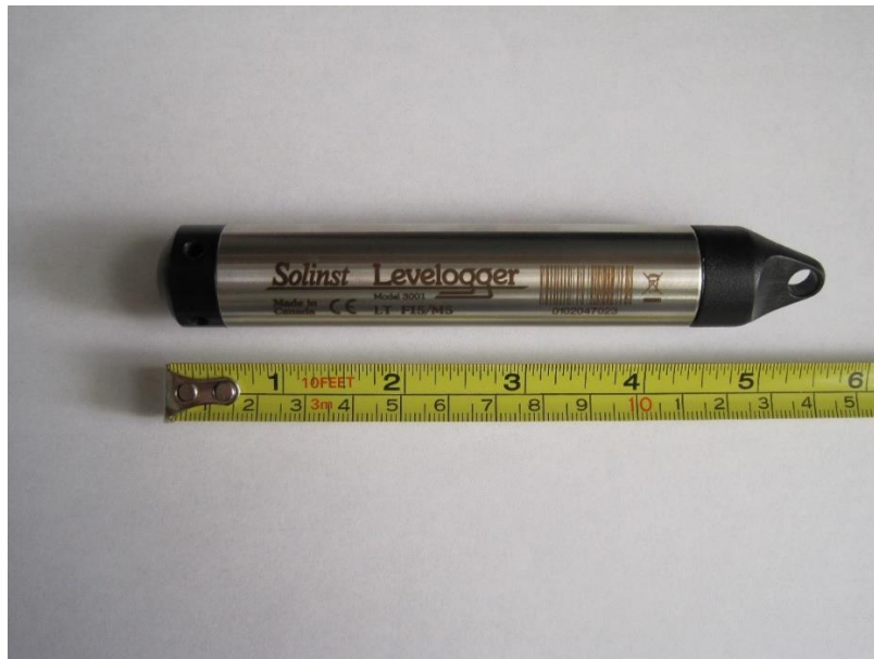
Figure 7- A Solinst levelogger used in the monitoring wells.
