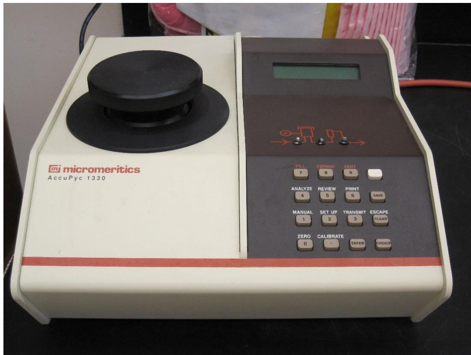
Figure 8: Accupyc 1330 Pycnometer used to measure porosity.
