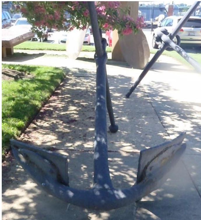
FIGURE 125. WNY018 bottom half showing converted flukes on the Washington Naval Yard (Marlowe 2015).
