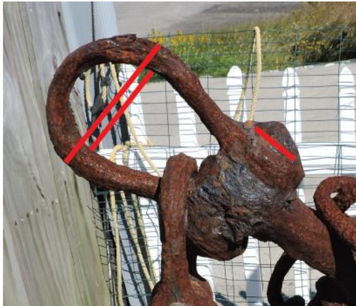
FIGURE 41. WNC005 showing the shackle diameter, shackle eye diameter, shackle pin thickness, and shackle opening measurements (Marlowe 2016).
