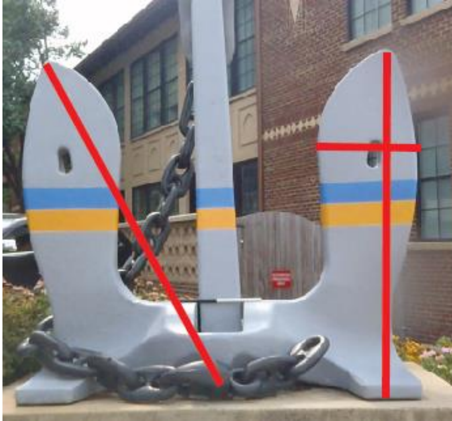
FIGURE 47. WNY009 showing one arm length, fluke length, and fluke width (Marlowe 2016).
