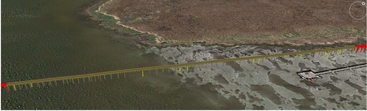
Figure 5.31. 3D virtual model created using existing wharf piles in Rhino 5 overlaid on Google Earth image (B. Scott Rose 2017).
