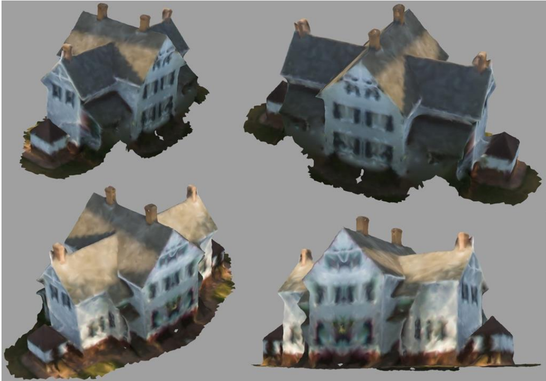
Figure 5.20. Virtual 3D Model of the big keeper's house at the CBLs, rendered in Agisoft Photoscan (B. Scott Rose 2017).
