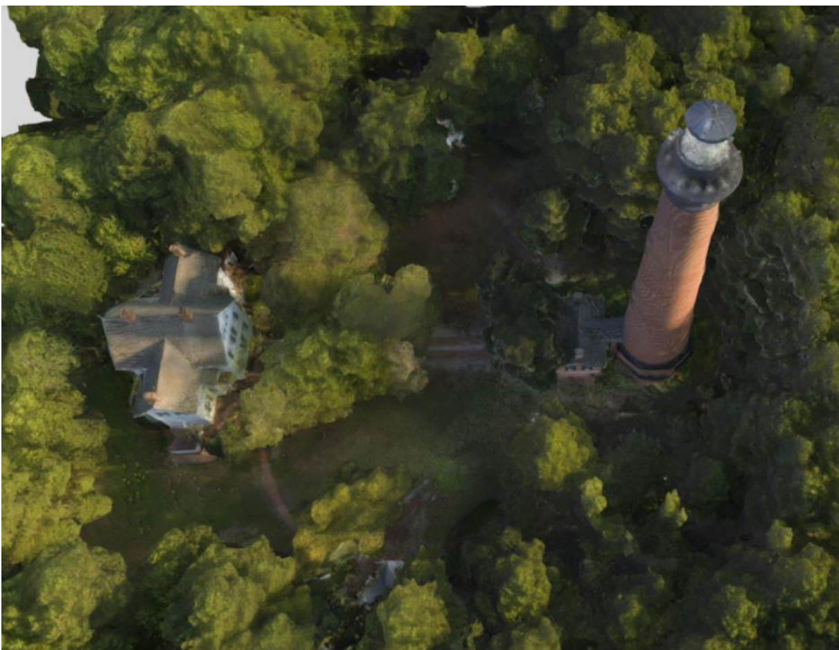
Figure 4.16. Photographic textures applied to wire frame model generated of CBLs over all complex using Photoscan . (B. Scott Rose 2017).
