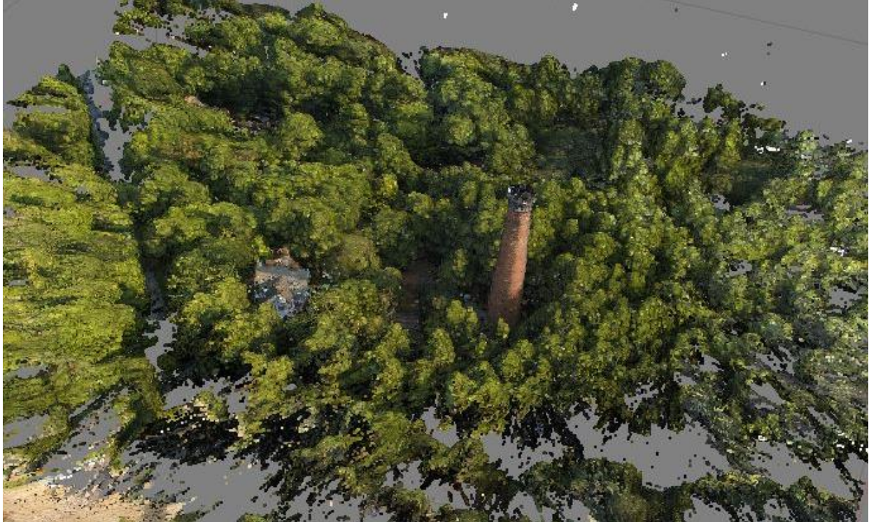
Figure 4.14. Dense point cloud generated of CBLS of the complex using Photoscan . (B. Scott Rose 2017).
