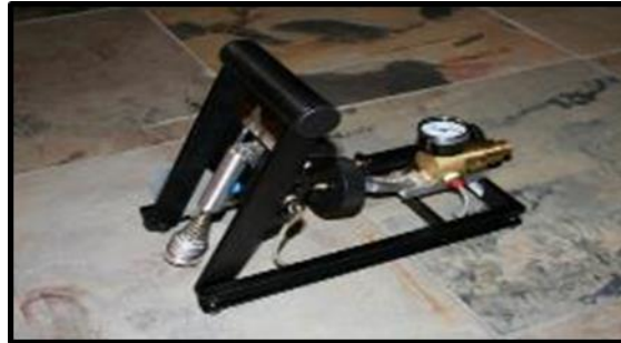
Figure 8- English XL variable incidence tribometer (Slip Doctors, 2017).
