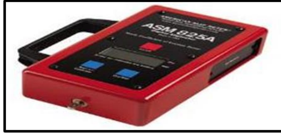
Figure 6- American Slip Meter ASM 825A manual drag sled (Slip Doctors, 2017).
