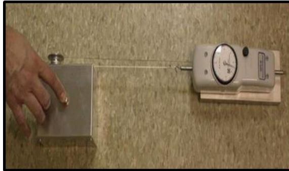
Figure 5- CSC force measurement horizontal pull slipmeter (C.S.C Force Measurement, 2017).
