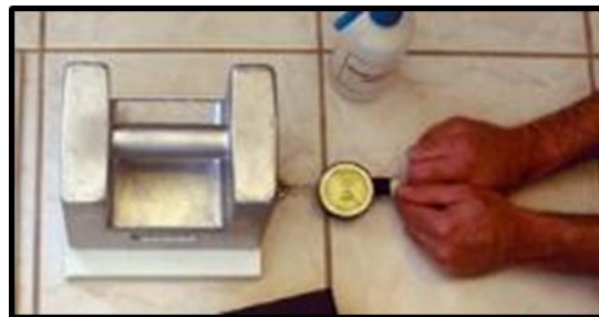
Figure 3- Horizontal dynamometer drag sled pull-meter (Slip Doctors, 2017).
