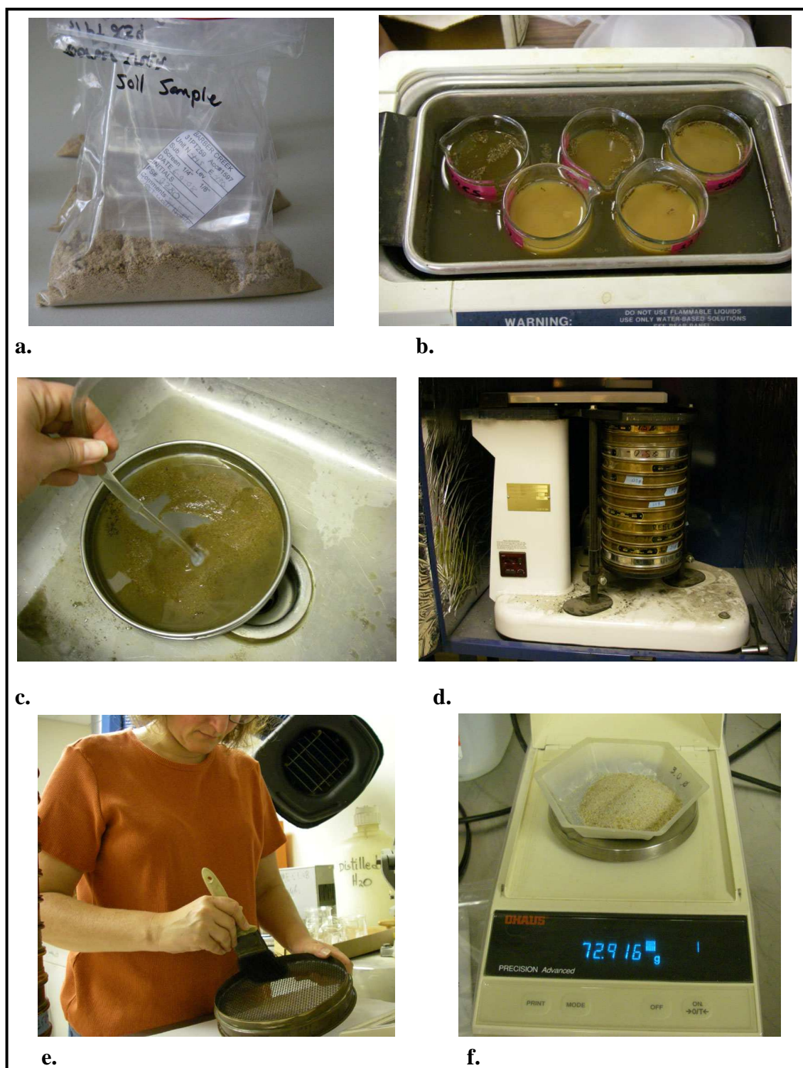
Figure 2.3. a) Sediment samples drying in bags. b) Sediment samples in sonicating unit. c) Washing sample to remove fines. d) Sieves in the Rotap machine. e) Sample being removed from sieve. f) Sediment sample being weighed.
