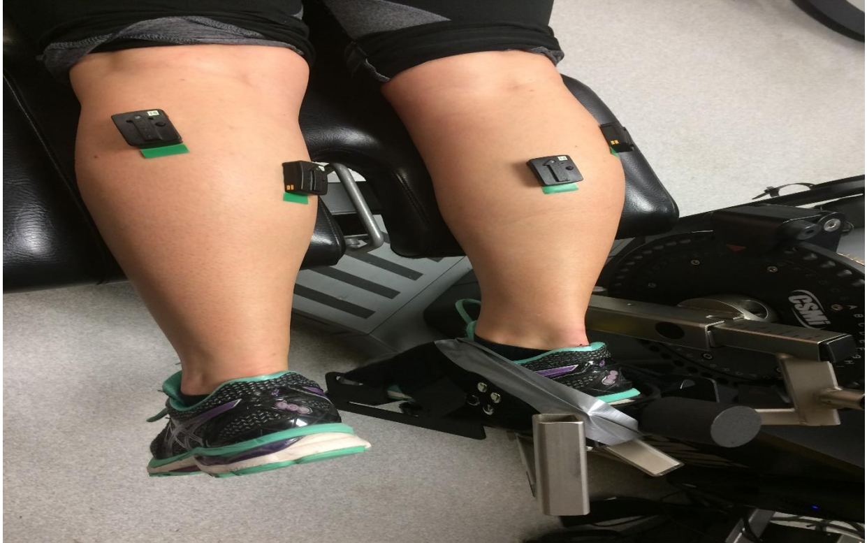
Figure 9: EMG electrode placement and dynamometer foot placement.
