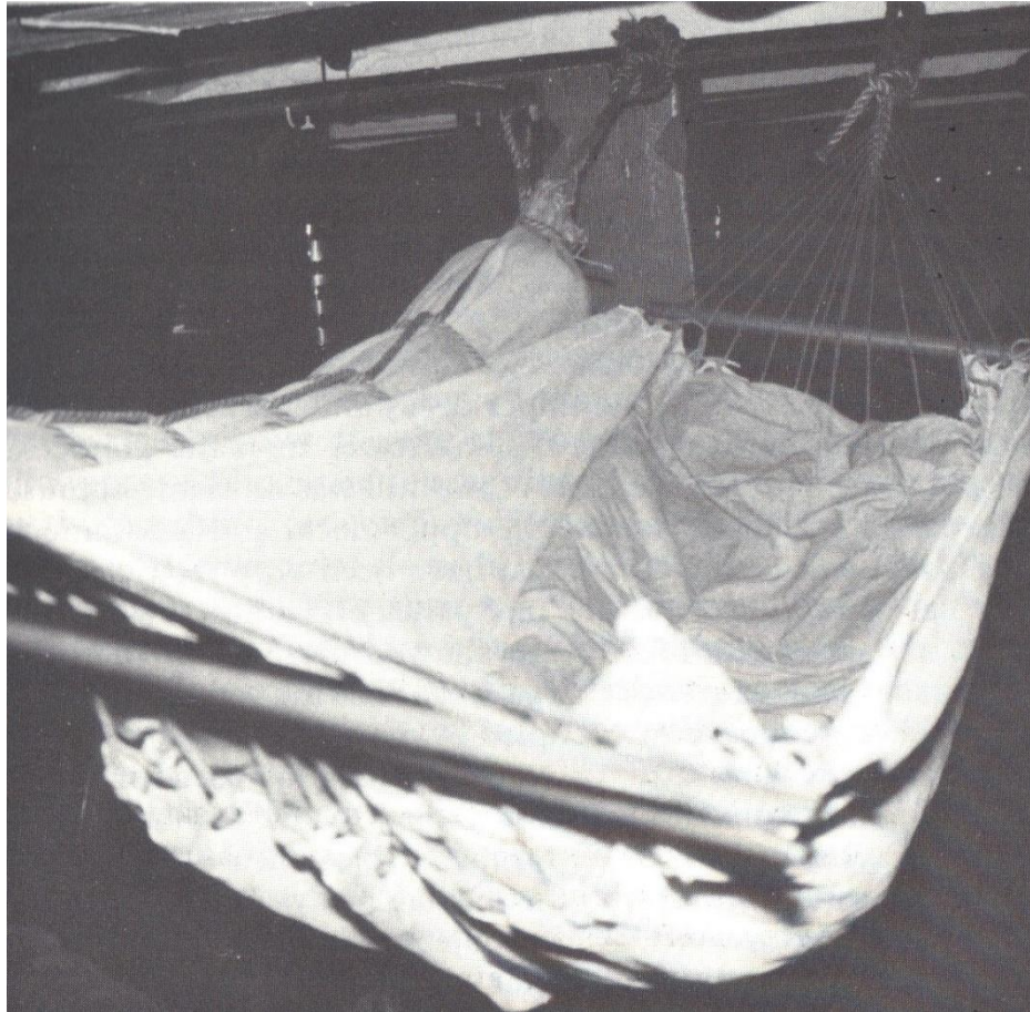
Figure 6. Slung hammocks with and without spreader bar, nettles and woven clews. Royal Navy, 1750's.
