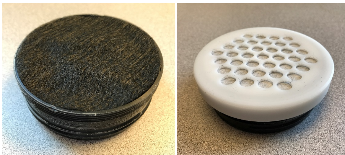
Figure 2. Respirator cartridge with 3-inch internal diameter and 1-inch bed depth: a) uncovered showing the ACF discs; b) covered
