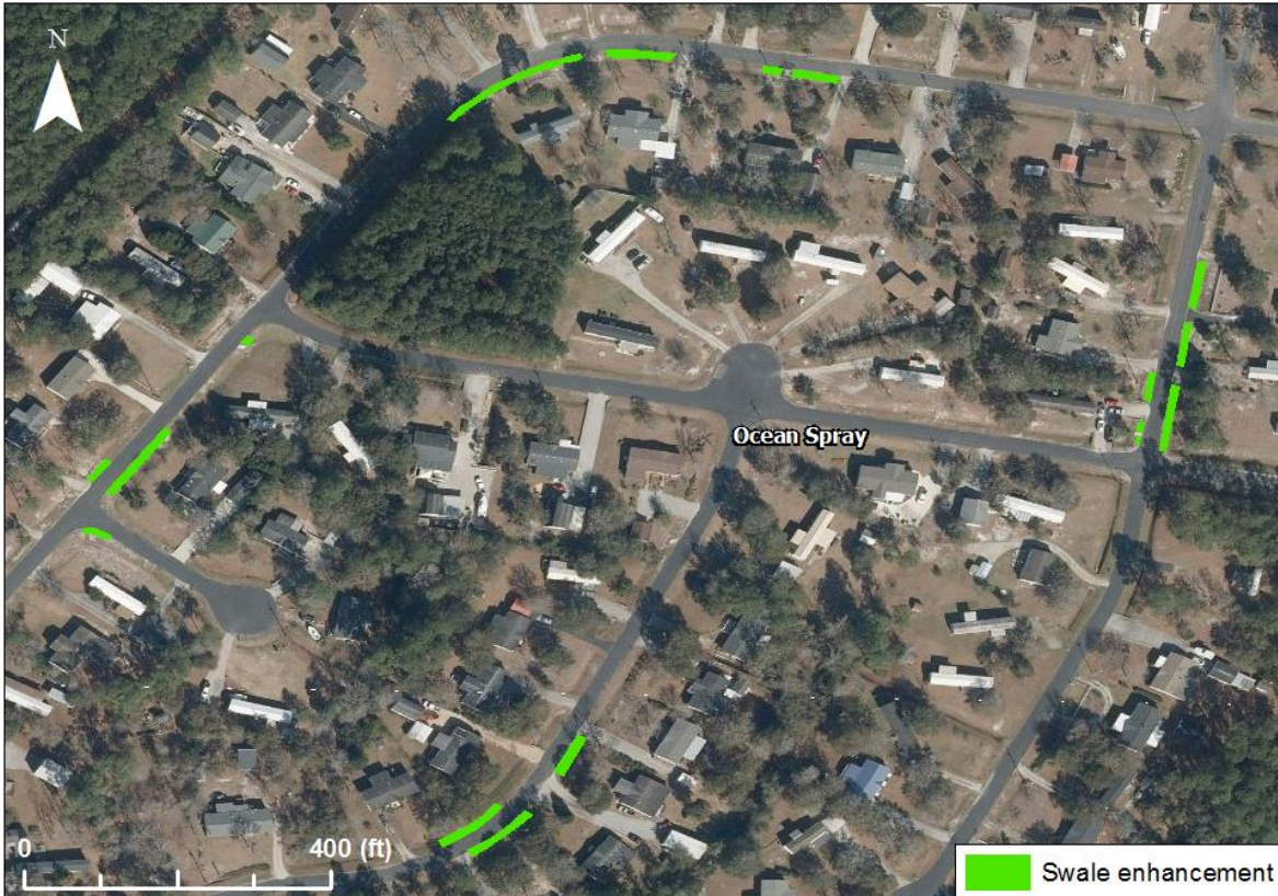
Figure 13. Locations of swale stabilization and enhancement in the Ocean Spray community. Enhancement location dimensions shown are approximated.
