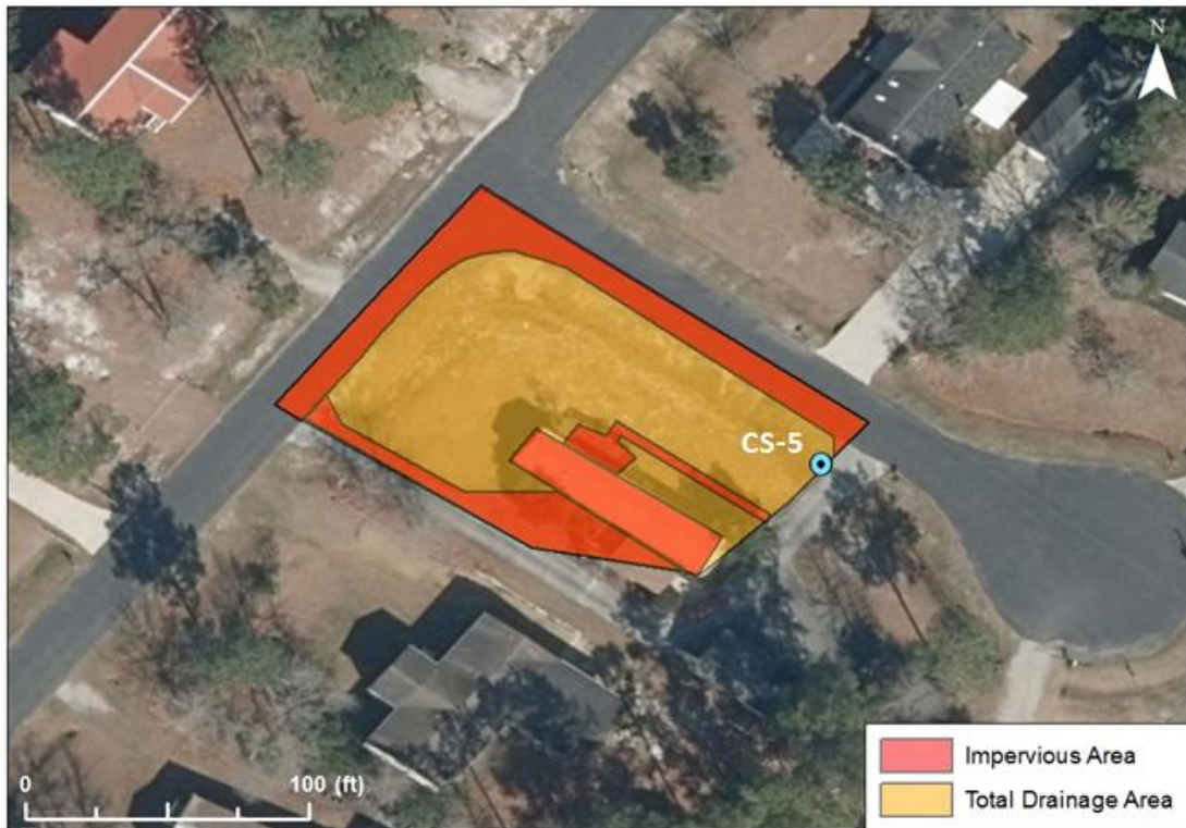
Figure 36. Total drainage area and impervious surface area for water control structure 5 in the Ocean Spray community.
