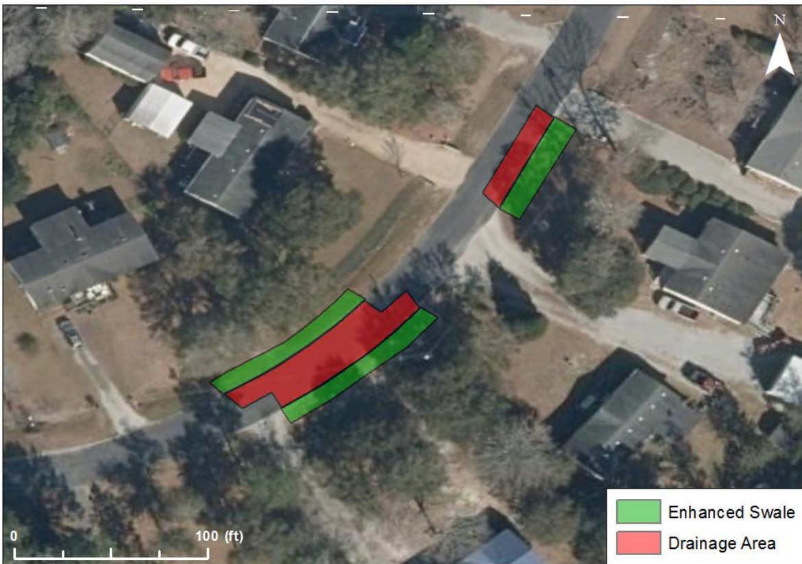
Figure 37. A portion of the enhanced swale drainage areas found within the Ocean Spray community.
