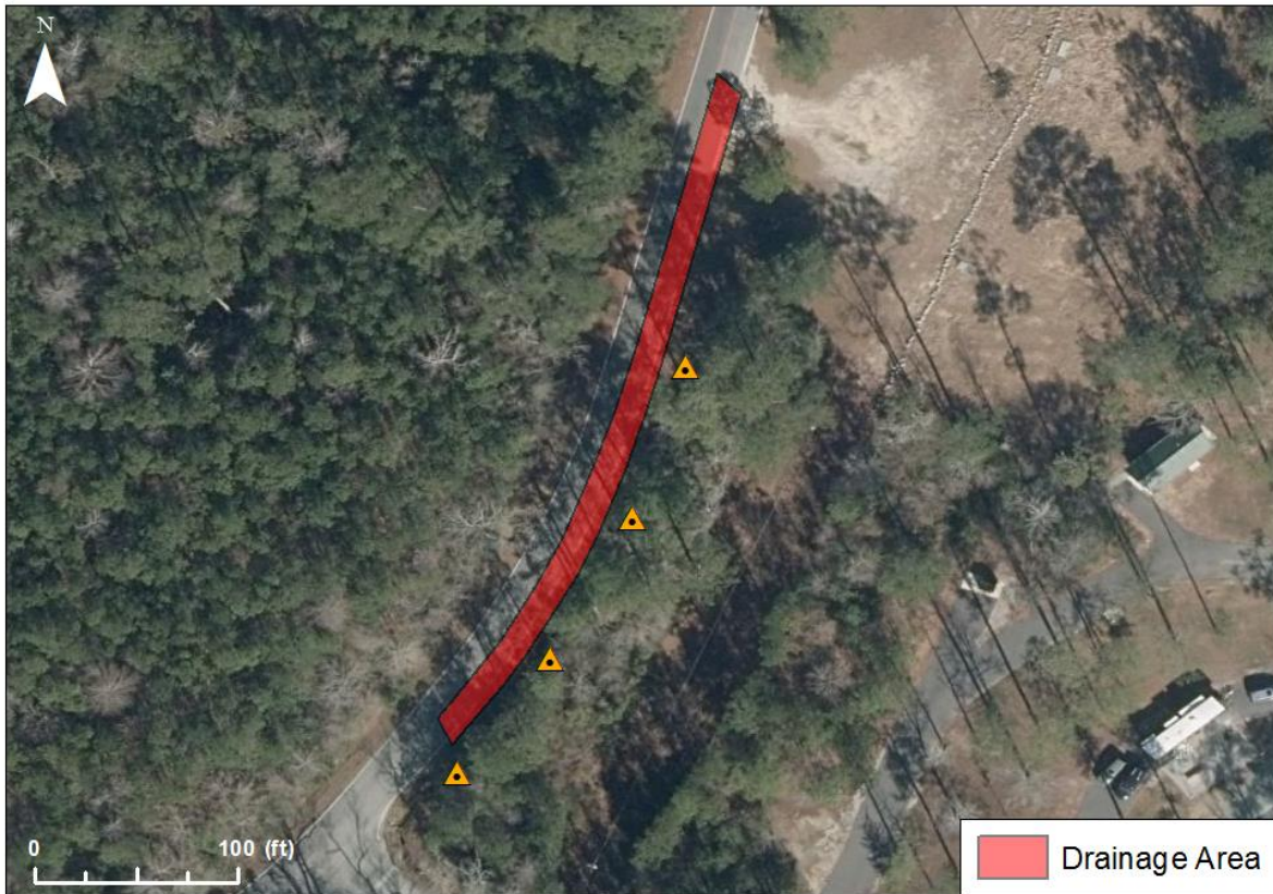
Figure 38. Drainage area for the rock check dams installed along Croatan Forest Road, near the Cedar Point Campground.
