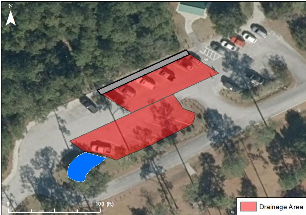
Figure 39. Drainage areas for the newly constructed walkway and rain garden at the Cedar Point Tideland Trailhead parking area and boat ramp.
