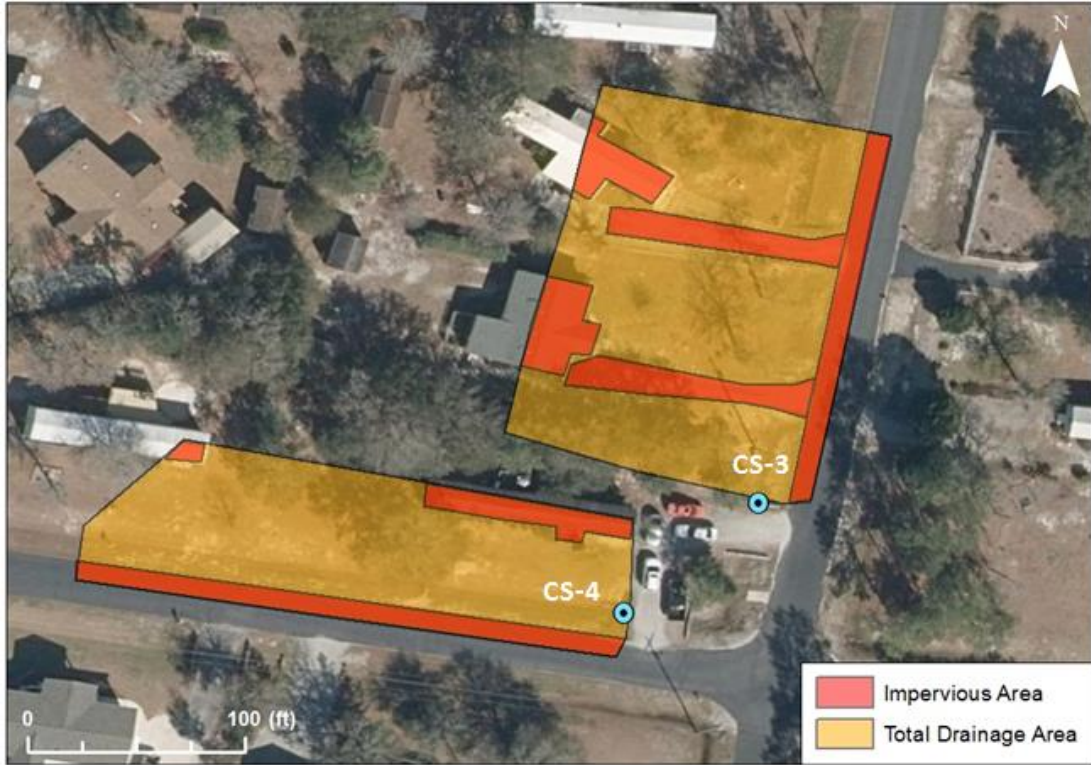
Figure 35. Total drainage area and impervious surface area for water control structures 3 and 4 in the Ocean Spray community.
