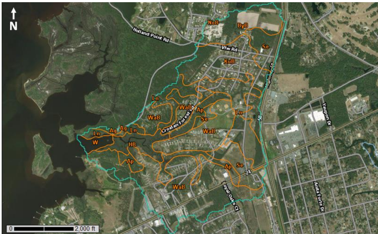
Figure 6. Soil map of the Boathouse Creek watershed (NRCS Web Soil Survey, 2016). Soils consist of predominantly sands to sandy loams. Explanation of unit symbols can be found in Table 3.
