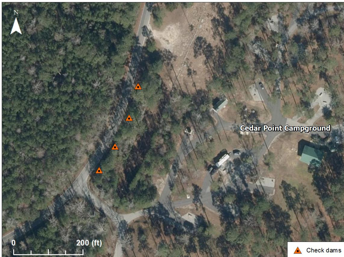
Figure 15. Locations of rock check dams installed along Croatan Forest Road, near the Cedar Point Campground.
