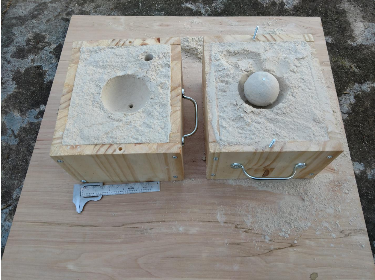
FIGURE 9. Salted sand core in the casting void. (Photograph by author).
