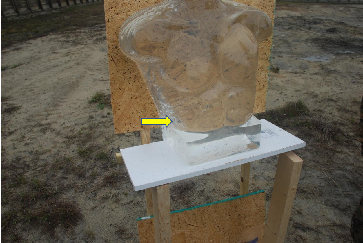
FIGURE 11. Glass shrapnel in ballistic gelatin torso lower right abdomen. (Photograph courtesy of L. Babits).
