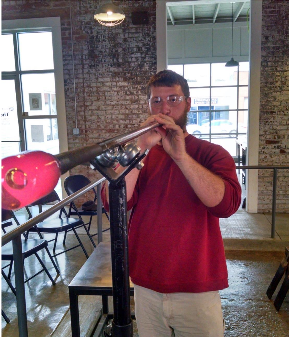
FIGURE 6. Creating the air bubble in the glass shell. (Photograph courtesy of Michael Tracy).
