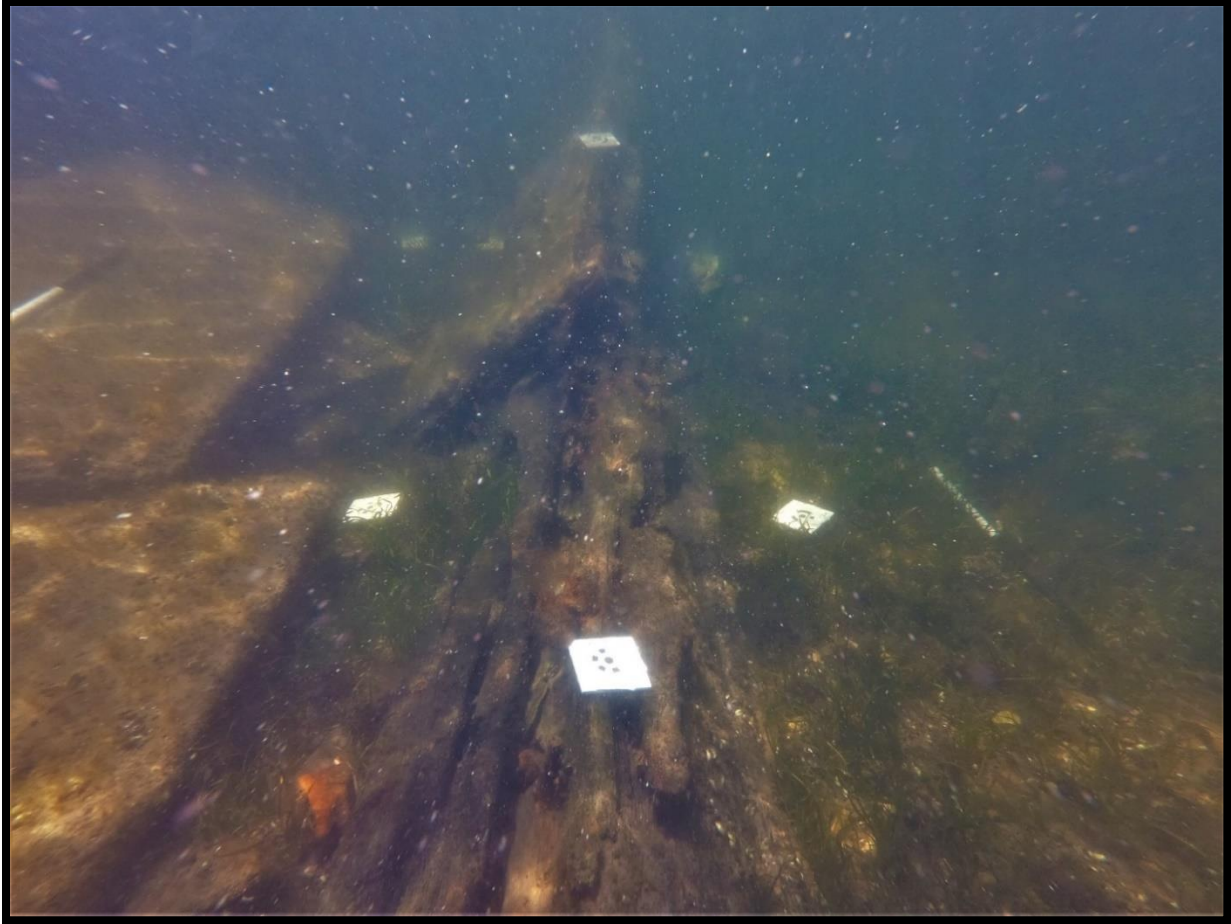
FIGURE 4.4. Coded targets and scale bars on the upside-down section of Excelsior 's stern (Image by Paul Willard Gates).
