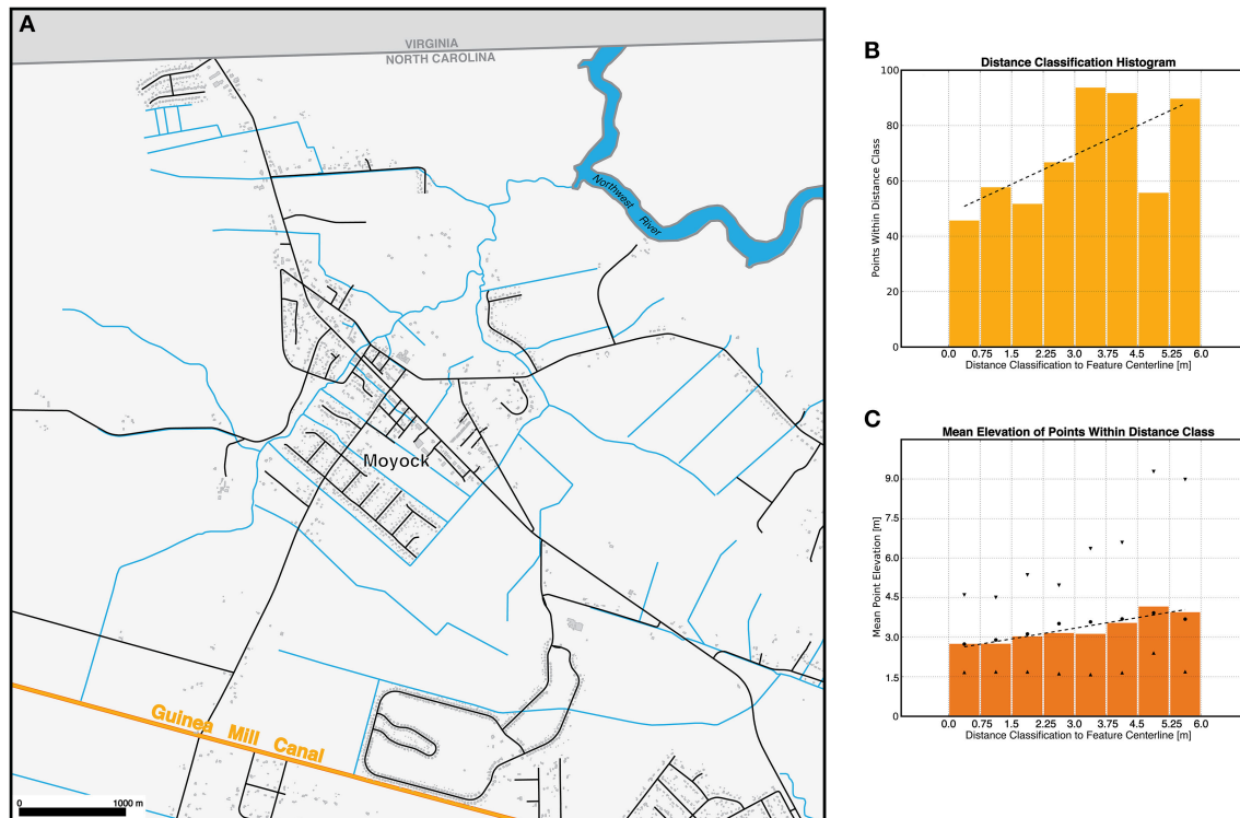
FIGURE 3 | Map inset (A) depicts a subset area of Moyock including all ditches, canals, and riverine hydrography (blue), roads (black), and buildings (grey) with the large Guinea Mill Canal highlighted to illustrate subsequent LiDAR point and buffer analyses; inset chart (B) histogram shows the number of points (y-axis) vs. multiple buffer distances of the Guinea Mill Canal centerline (x-axis), an analysis that was conducted on all ditched features; and the chart (C) illustrates the elevation variation of LiDAR points with distance from the centerline of Guinea Mill Canal, highlighting a best-fit OLS regression relationship used in selecting an optimal buffer distance to preserve minimum elevation for attributing the ditch.
