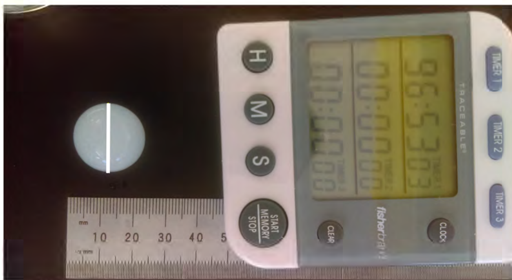
Figure 3.3: A super absorbent polymer bead imported into ImageJ with the line draw that measures the diameter.
