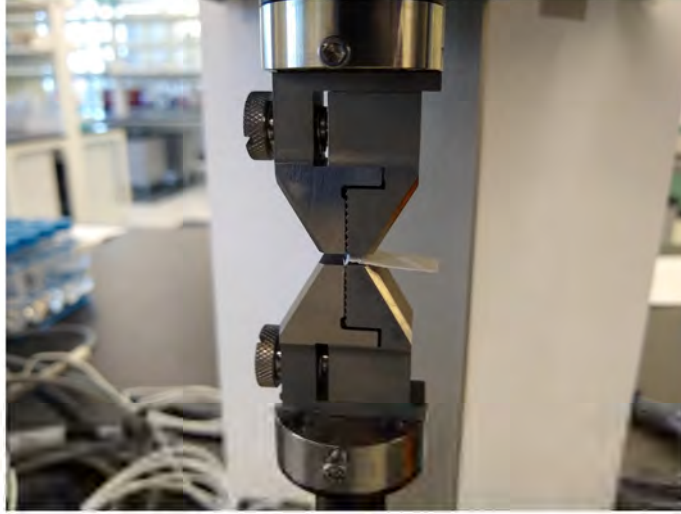
Figure 4.2: Setup for the electrospun fiber mat testing on the TA Electroforce 5500 with metal grips attached.
