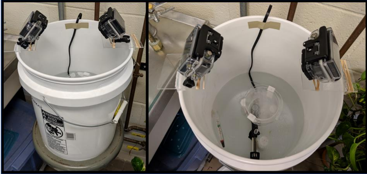
Figure 1. Behavior Trial Set up Includes: (1) trial bucket with two camera platforms, (2) plexiglass stand, (3) aquarium heater, (4) aquarium thermometer, and (5) two GoPro Hero3 Black Edition HD3.03.00) cameras (Photo by B. Gerald).
