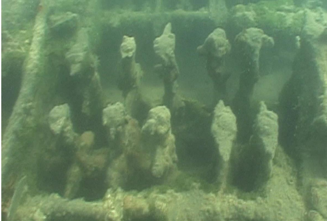
Figure 63. Fasteners that once held planking to the frames (Image from 2008 ECU archaeological survey).
