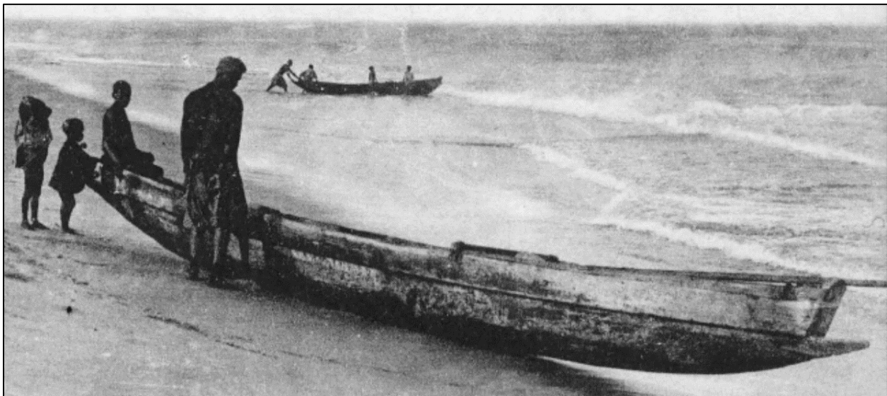
Photograph 4.3.15: Senegal River Coast boats with no extended cutwaters being launched Cropped, from (Tacher Unknown)
