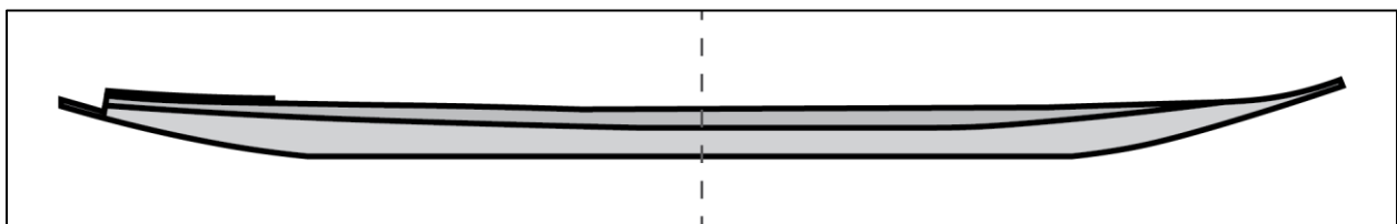
Figure 4.6.2: Gambia-Sine/Saloum extended logboat with projecting cutwater, Profile view Approximate shape from photographs
