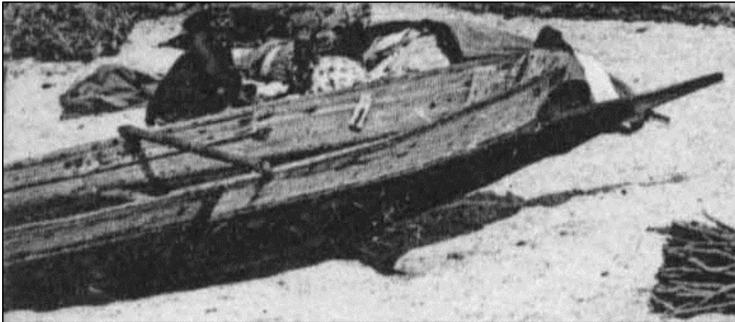
Photograph 4.10.5: Boat using small batten and uneven futtocks
