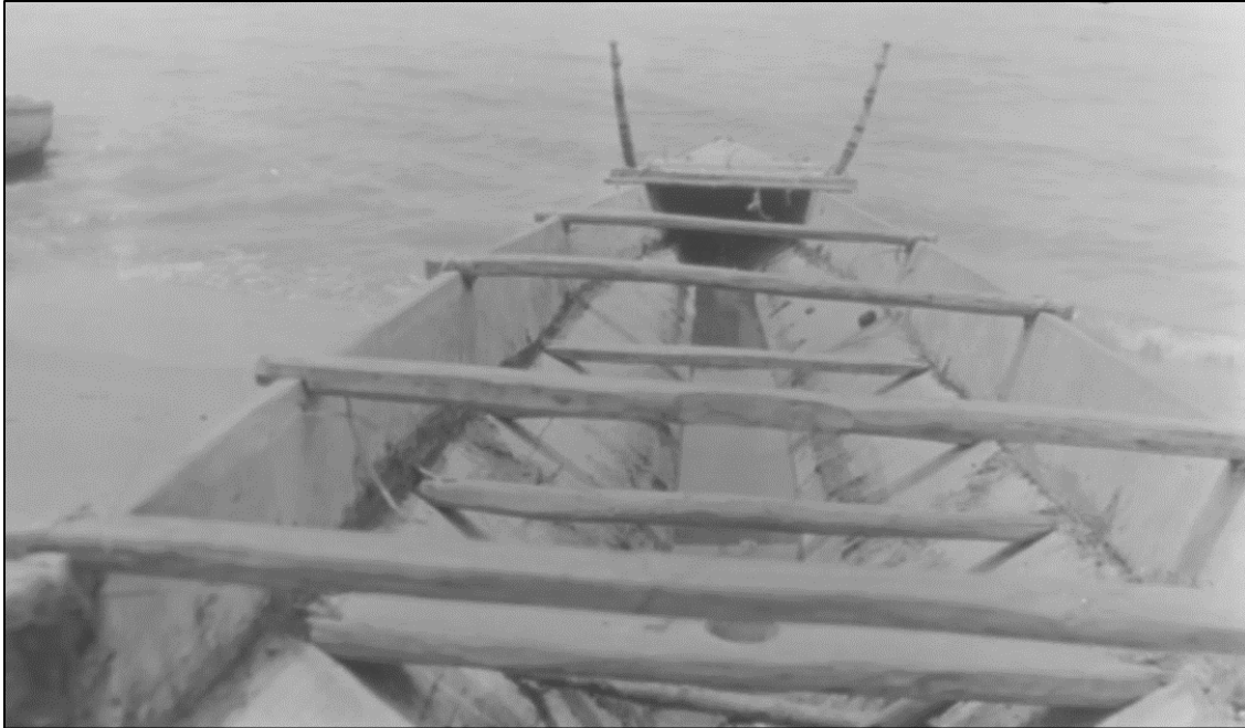
Photograph 4.12.2: Fore end and interior of a shell-based plank-built fishing boat showing thwart layout and mast thwart, Gambia Cropped, from (Hornell 1928d)
