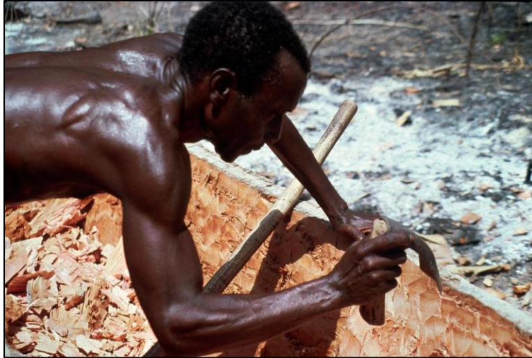
Photograph 4.9.9: Smoothing the Inside of a logboat, Senegal From (Petersohn Unknown)
