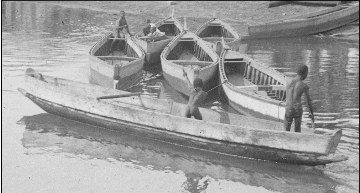
Photograph 4.3.16: No extended cutwater boat with reinforced front, likely a coastal boat, appeared to be nailed construction Cropped, from (Tignol 1900)
