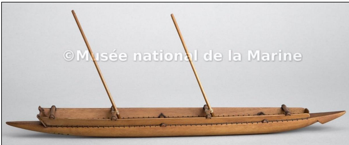
Model 4.13.1: Model of an 1830 boat from the Cape Verde Peninsula, likely mounted a lugsail From (François 1873) Model made from direct measurements of a boat and overseen by someone who observed the boats firsthand although significantly after initial measurements and observations.
