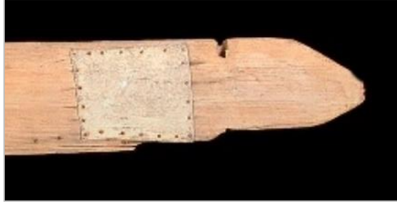
Photograph 4.19.2: Lead plate attached to a steering oar from the Cape Verde Peninsula
