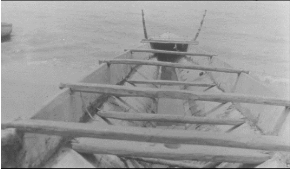
Photograph 4.10.2: Fore end and interior of a shell-based plank-built fishing boat, Bathurst Gambia
