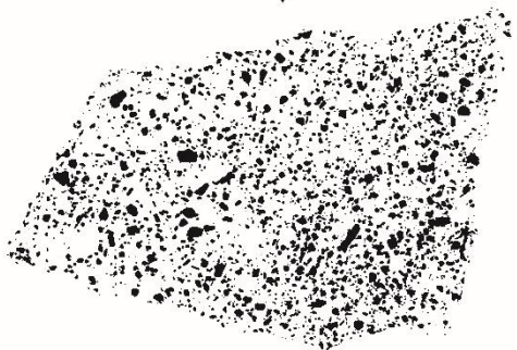
Figure 32. A. Rock slab image of sample ME12 analyzed for CSD of plagioclase phenocrysts. B. Resulting photoshop image after isolating crystals based on color. C. Resulting ImageJ photo after removal of image parts of 5 pixels or less and after filling in missing area of crystals and removal of incomplete crystals around edges D. Produced CSD curve for sample ME105.
