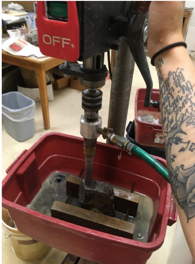
Figure 30. Drill used for coring all samples to extract 25-mm diameter cores.
