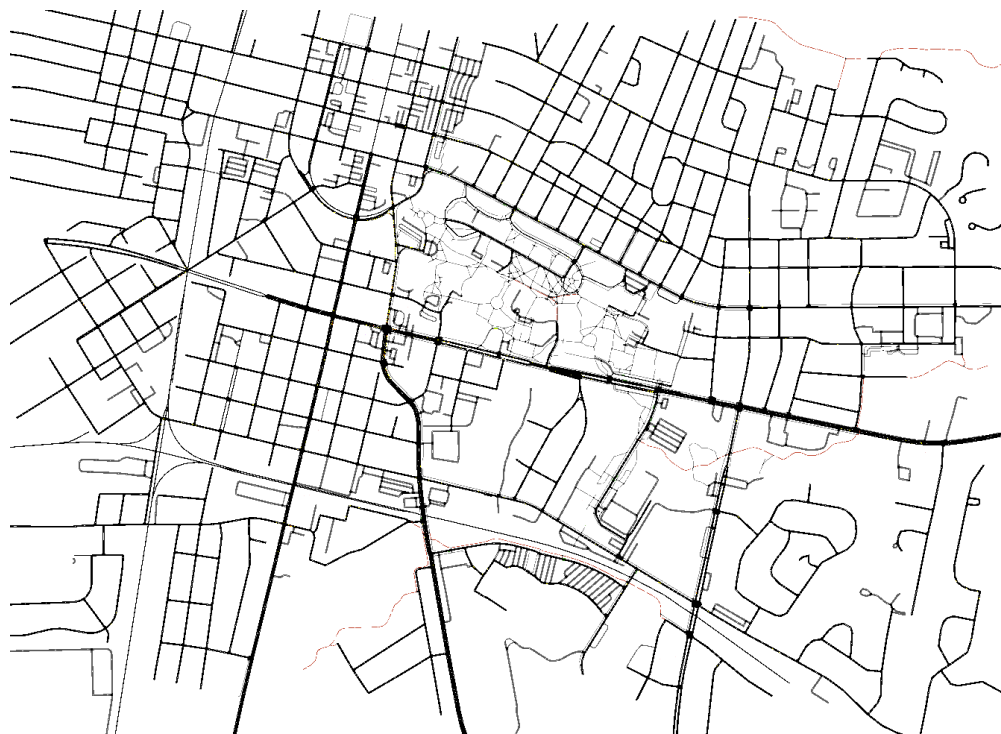
Figure 2.1: Subsection of Greenville, NC Traffic Network in SUMO
