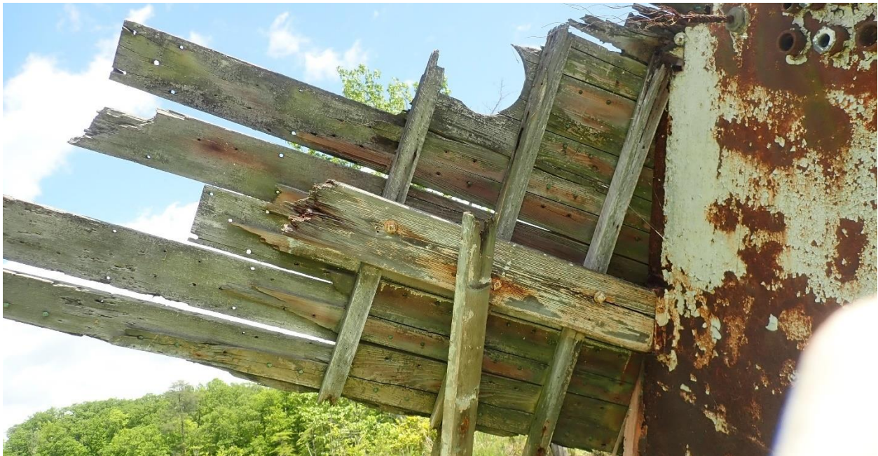
FIGURE 6.27 The interior of the outer hull planking behind Bulkhead 6 of the Sea Scout Wreck showing areas where the lignin in the wood has not yet broken down, but algae growth is present (Photo Credit: Nathan Richards, 2021).
