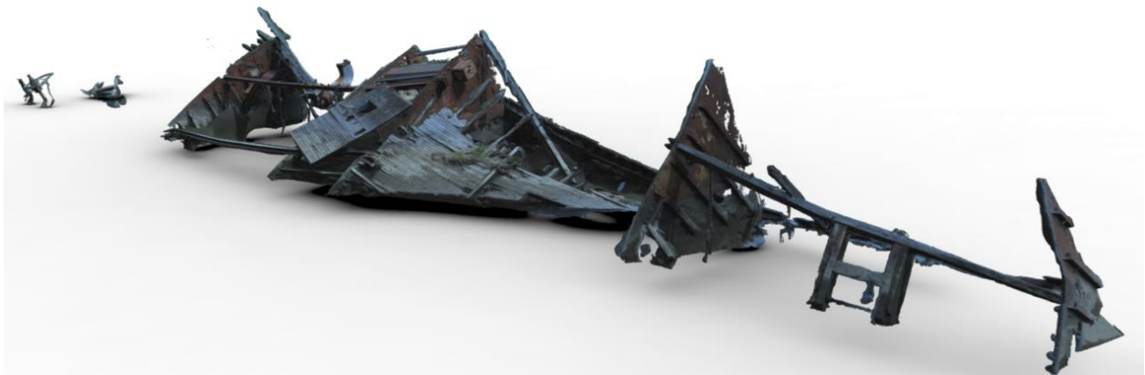
FIGURE 6.17 Photogrammetric Model of Sea Scout showing the most accurate positions of the bulkhead of the Sea Scout Wreck (isometric view) (Model created by Nathan Richards).
