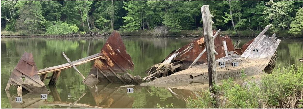
FIGURE 5.13 Picture of the Sea Scout Wreck showing the locations of bulkheads B1 through B6, B7 is present at the site but is not visible in this image (Photo credit: Frances Park, 2021).
