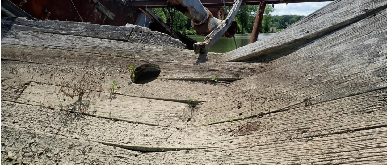
FIGURE 6.26 The port side hull of the Sea Scout Wreck in 2021 showing the grey-silver discoloration associated with the breakdown of lignin in the wood (Photo credit: Nathan Richards, 2021).
