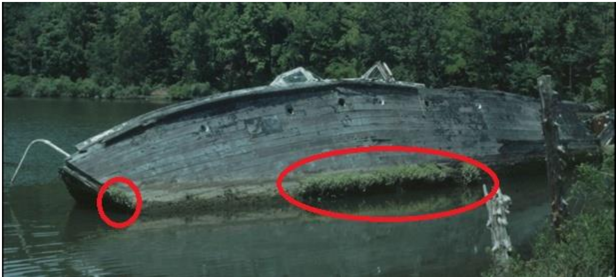
FIGURE 6.25 Port side of the Sea Scout Wreck in 1997 showing plant grown on the hull (circled in red) at the water level (Photo courtesy of Susan Langley, 1997).
