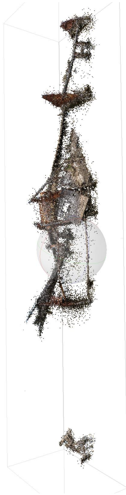
FIGURE 3.23 The sparse cloud showing the camera tie points for the aligned photos (Image by Taylor Picard, 2021).
