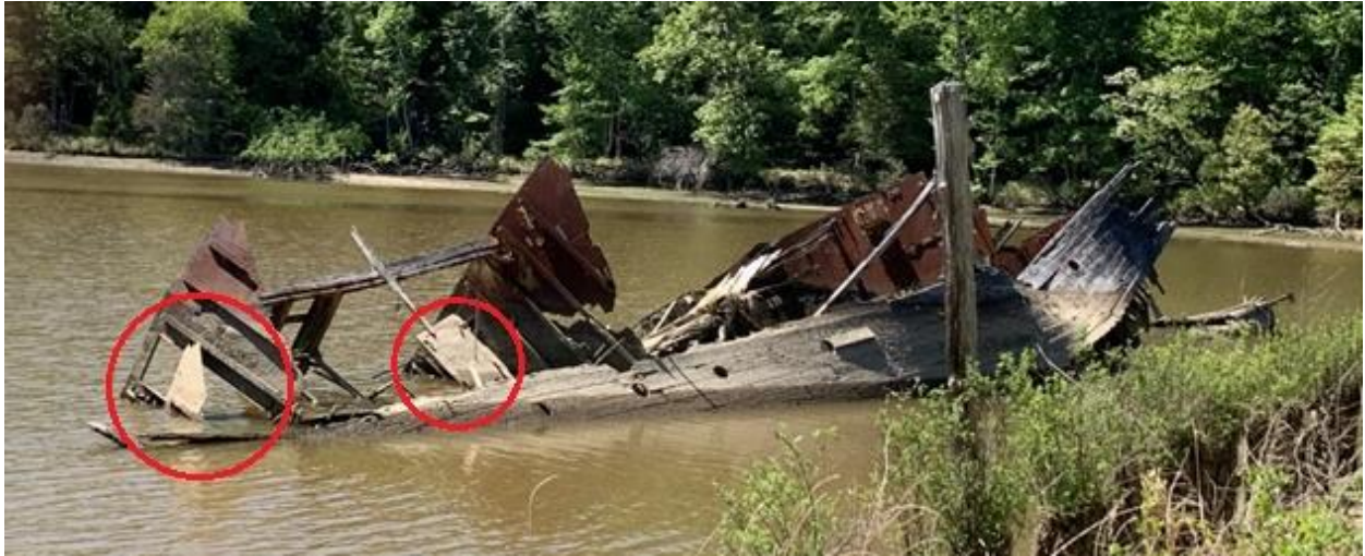
FIGURE 5.5 The Sea Scout Wreck with low water levels, revealing the bulkhead doors (circled in red) (Photo Credit: Frances Park, 2021).
