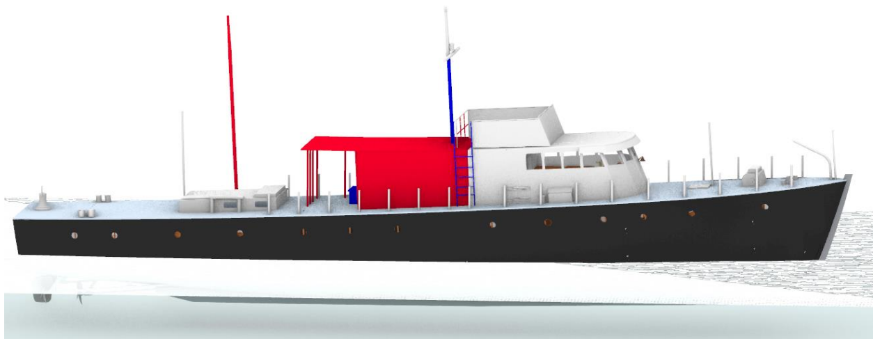
FIGURE 6.7 Alexandria 104' ARB (1976) showing the features that were altered in blue and added in red (Model created by Taylor Picard).
