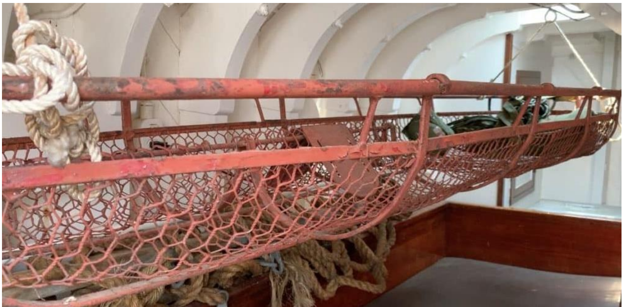
FIGURE 5.20 Pipe Berth from P-520, an 85' ARB that now operates as a floating museum ( Chesapeake Magazine , 2021).
