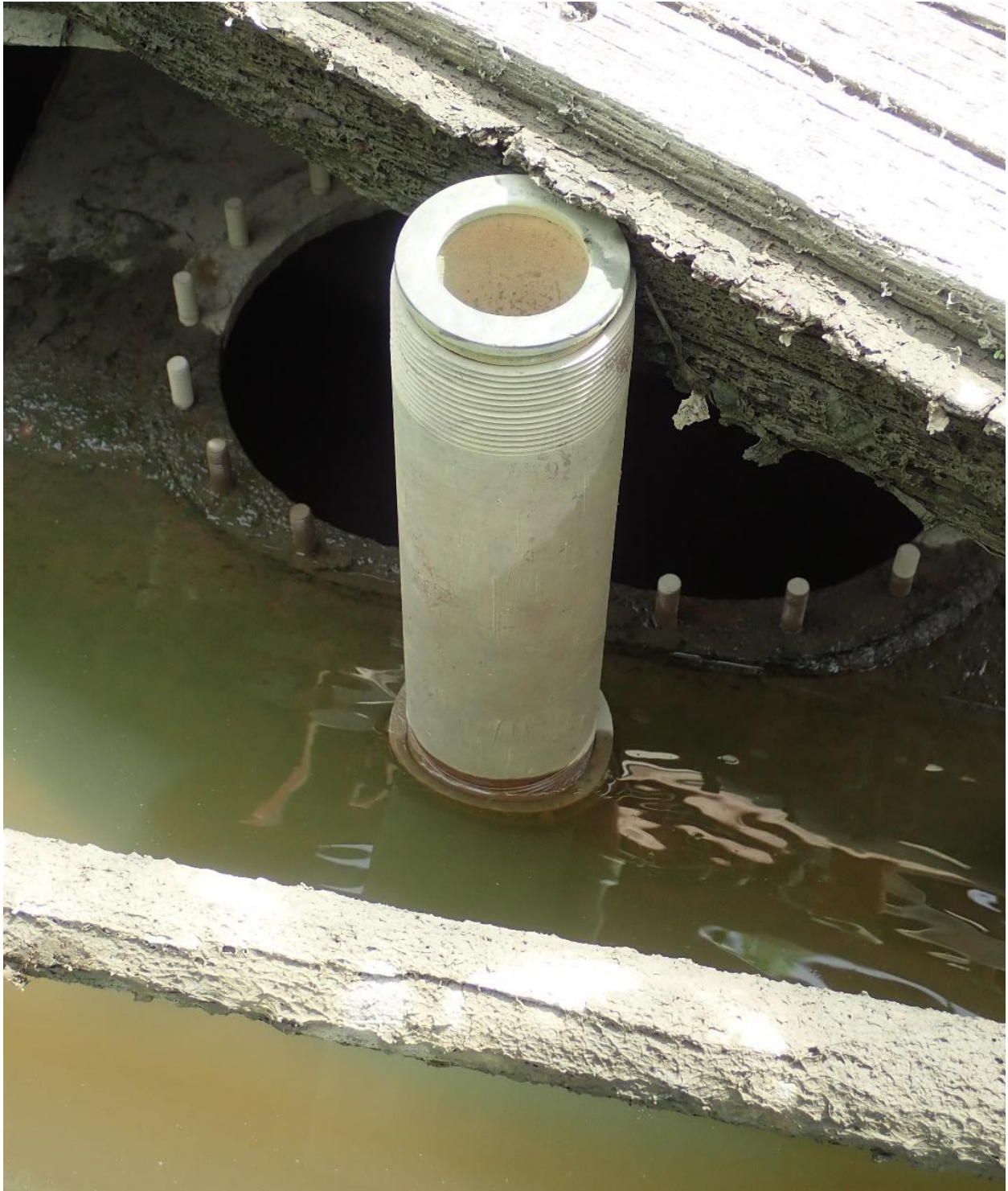
FIGURE 6.13 PVC pipe mounted to the top of the starboard fuel tank of the Sea Scout Wreck (Photo Credit: Nathan Richards, 2021).
